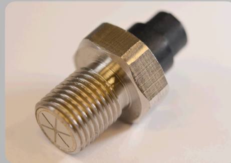
Power cartridge replicator: low cost output replicator designed and produced for WFO development (modified bolt to match mechanical interface).
