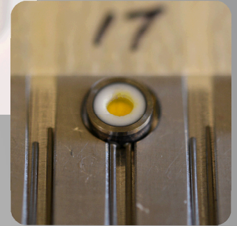
Power cartridge replicator: low cost output replicator designed and produced for WFO development (modified bolt to match mechanical interface).
