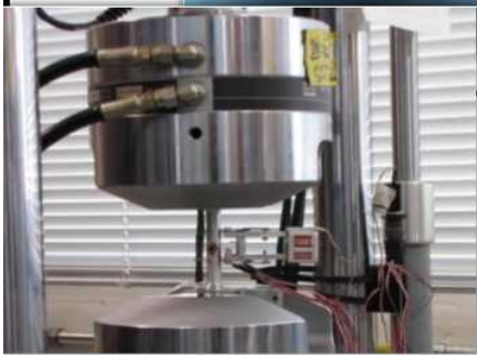
Standard cylindrical test specimen instrumented with strain gages and an extensometer walled tubes
