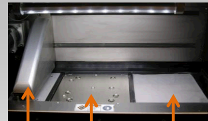
Recoating Blade Build Platform Dispenser Platform Powder Bed
