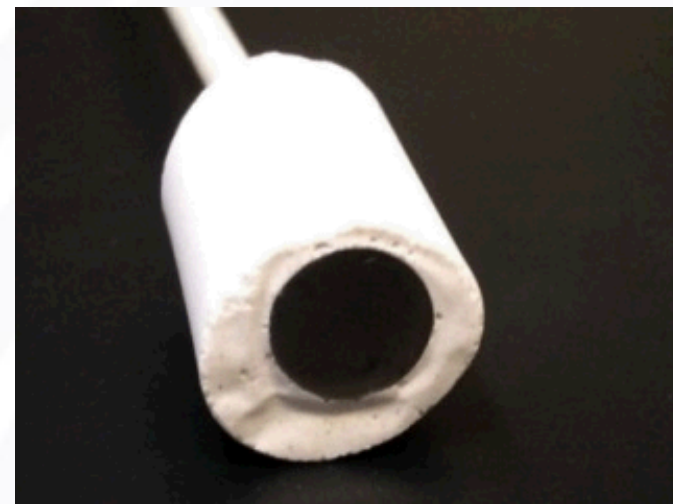
Encapsulated 347SS cylinder
