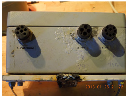
Figure 31. This enclosure has suffered severe water damage from a small nick in the connector o-ring. When the connector holes are drilled, the powder coat is broken. Normally, the receptacle o-ring prevents water getting into the break. After two years on a NOAA ship, salt water penetrated under the damaged o-ring and under the powder coat finish. Extra care is taken to assure the o-rings are perfect and a sealant is used to further protect the box.
