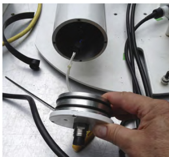
Figure 21. Carefully remove the endcap. Unplug the in line connector to free the endcap.
