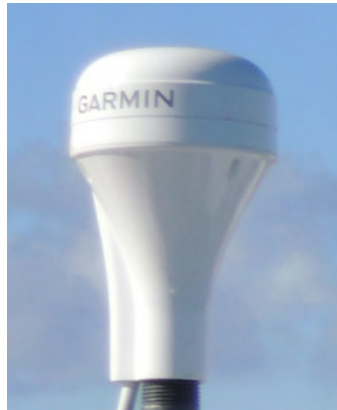
Figure 11. The Global Positioning System (GPS) receiver is a Garman Model GPS17X. The all-in-one unit is programmed to operate at 1-Hz NMEA0183. The NMEA0183 record includes UTC, position, SOG, COG, and magnetic variation.
