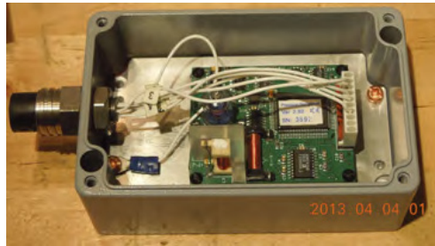
Figure 12. The TCM is the Precision Navigation Inc. Model 2.5. The serial output format includes pitch, roll, flux-gate compass, board temperature, and three components of earth magnetic field. The TCM sensor is located on the FRSR plate and the tilts are used to determine the tilt of the MFR head.
