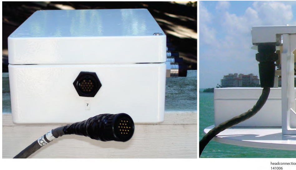
Figure 4. Connection to the MFR head is delicate and must be made with great care.
