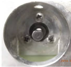
Figure 23. Align the motor shaft so the flat surface is pointing toward the access hole.
