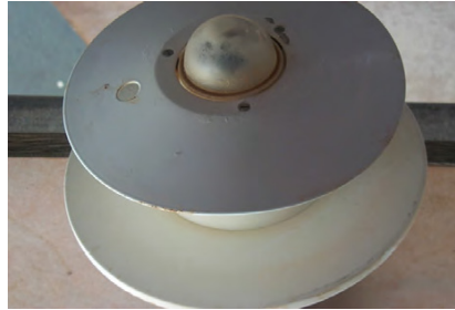
Figure 29. An accumulation of dust on a PSP from the Saharan desert. The radiometer was on a ship operating in the Caribbean Sea and the deposit came across the Atlantic Ocean.
