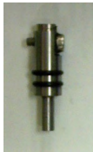
Figure 25. Shadowband shaft assembly. The set screw is at the top left and nadir magnet is on the right. The o-rings should be smooth and in good condition.
