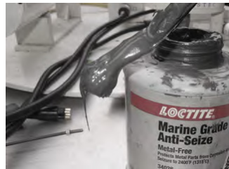
Figure 27. Anti-seize is messy but is essential for exposed hardware, especially for dissimilar metals such as for stainless bolts in aluminum.
