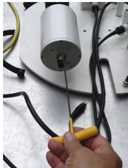
Figure 20. Unplug the motor cable and unscrew the four screws using a 3/32" Allen wrench.
