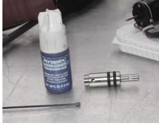
Figure 26. Blue LokTite is very strong but the set can be broken with ordinary tools. It is best for all set screws.
