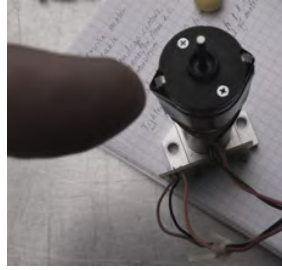
Figure 22. Connect about 5 VDC to the terminals of the motor. A voltage of 5-12 V can be used, but the motor turns more slowly with smaller voltage and thus is easier to align.
