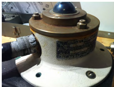
Figure 30. The PIR in this image was left unattended for several months on a tropical island in the Indian Ocean.
