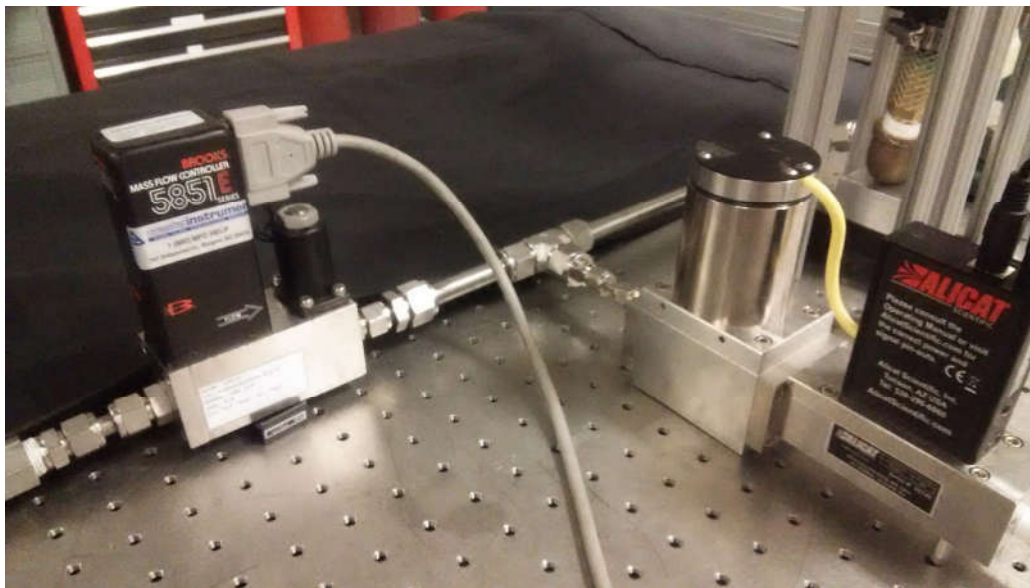
Figure 7: Forced Draft Ring-Stabilizer Air Pre-Mixing Manifold
