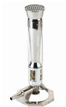
Figure 13: Picture of Fisher burner
