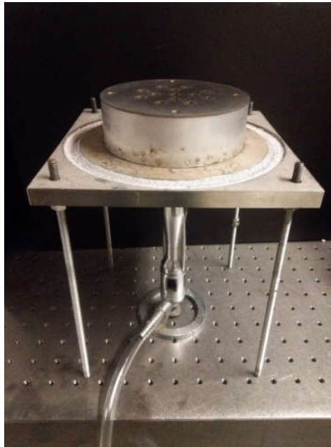
Figure 15: Natural Draft Ring-Stabilizer Fuel Venturi Assembly
