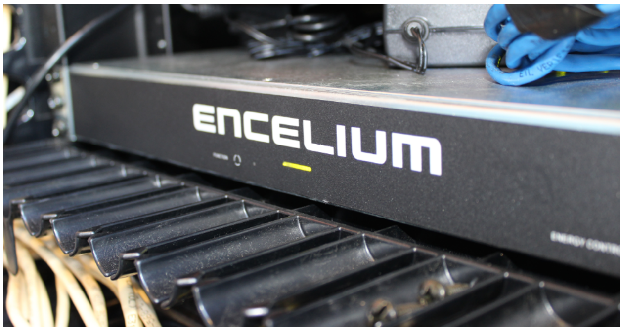
Figure 4.1 - Encelium's Rack mounted Energy Control Unit (ECU)
