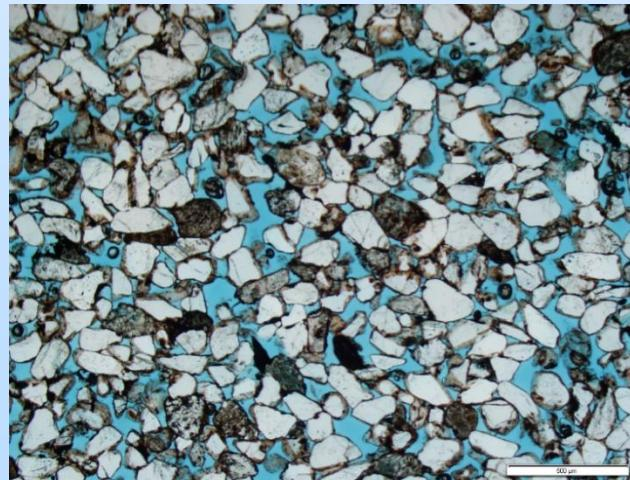
Lower Mt. Simon can have up to 30% porosity. Porosity largely secondary via feldspar dissolution.
