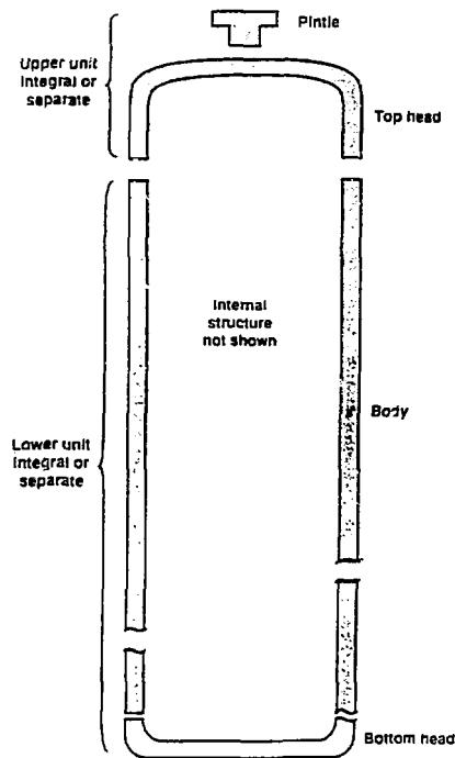
FIGURE 1 - Possible Container Components
