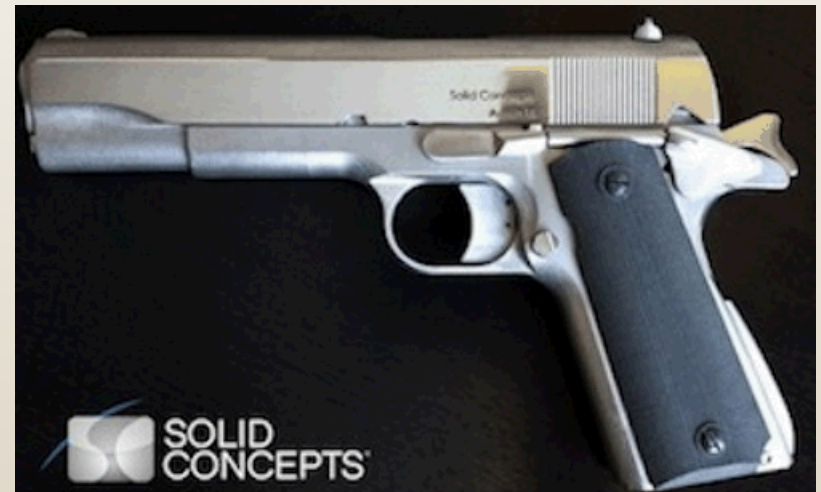
1911 .45 semi-automatic pistol fresh off the 3D printer, 2013, Stratasys Direct Manufacturing
