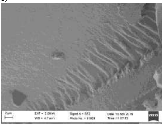
Figure 96. a) Image of the copolymeric material; b-f) SEM images of pure kraft lignin (b), and copolymeric material - top view (c,d), fracture line (e,f).
