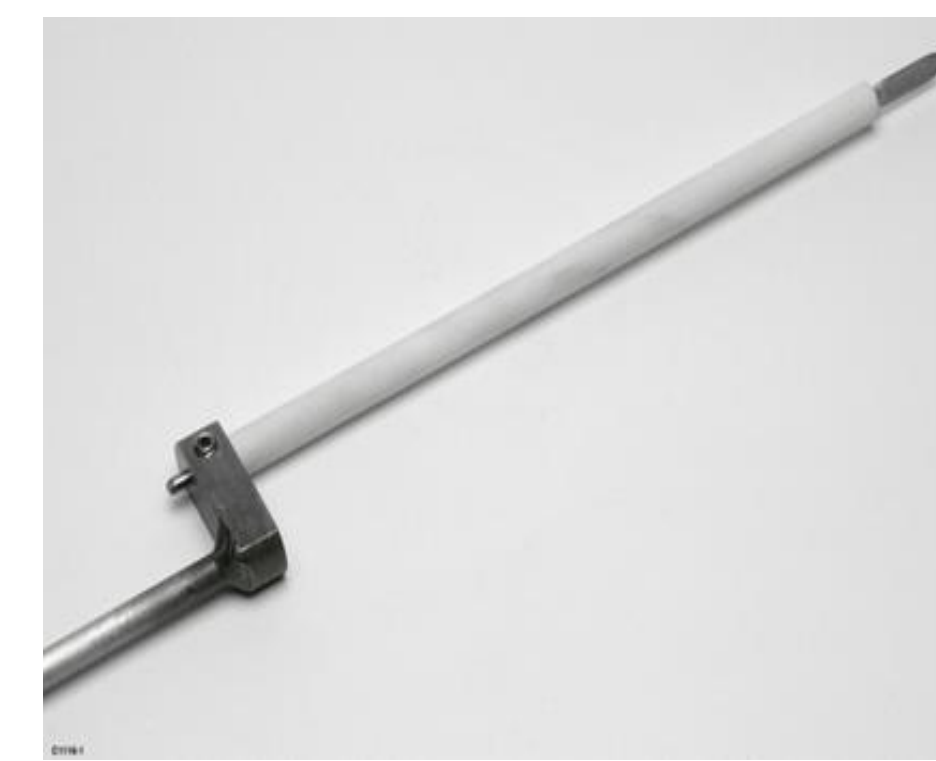
Figure 8: ER Anode is lowered into the inner portion making electrical contact with the impure metal.
