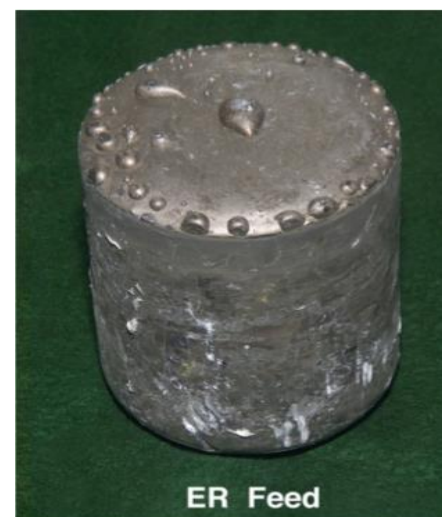
Figure 3: Feed Metal before ER
