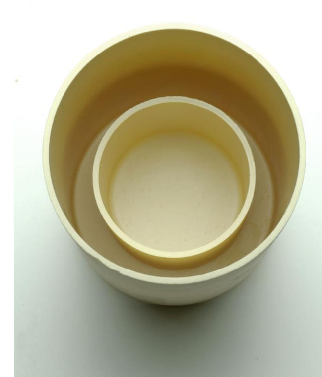
Figure 6: ER Crucible, shows the inner section Cathode, suspended above outer (impure Pu), and outer section (pure Pu)
