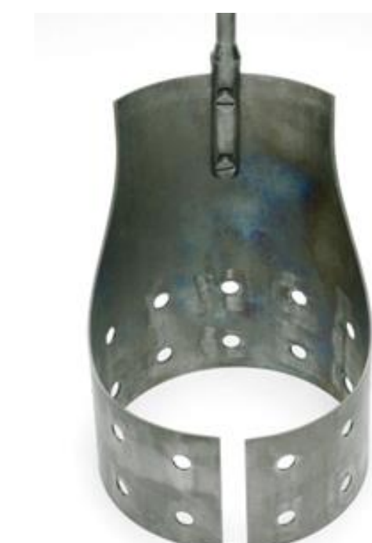
Figure 7: ER (Tungsten) shows the inner section Cathode, suspended above outer portion of crucible to allow purified Pu to drip down.
