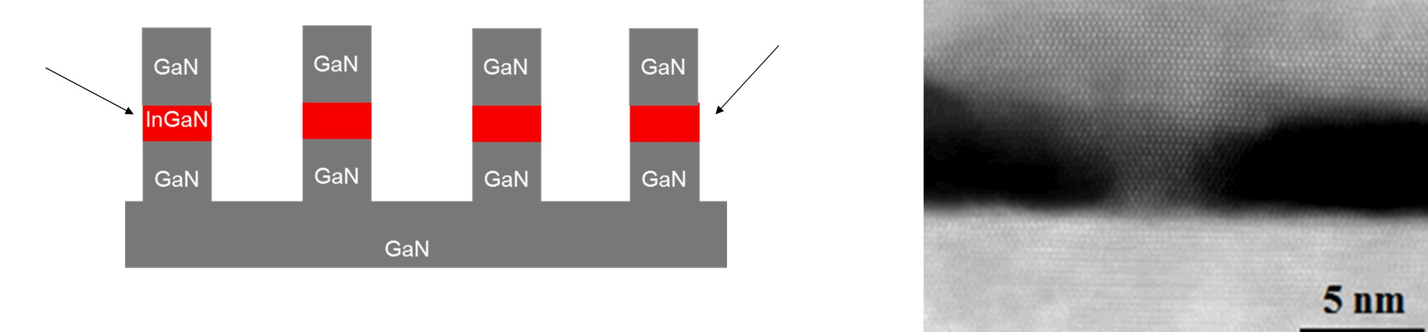
Multiple QDs from microfabricated nanowire arrays
