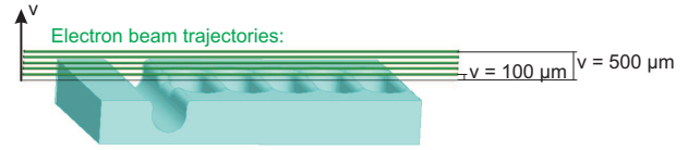
Figure 18: Vertical relative position of the beam with respect to one half of the structure.
