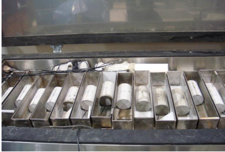
Figure 9 Cylinders in the freeze thaw machine
