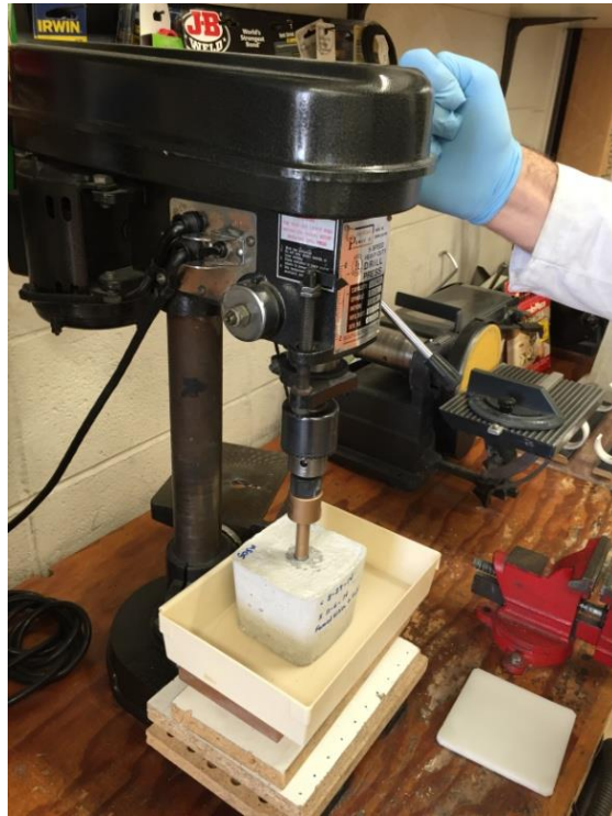
Fig. A-71(a) Diamond studded drill ( \text{Ø } \frac{1}{2} " DAMO). (b) Drilling into a concrete block using a drill press, process carried out over a plastic tray.
