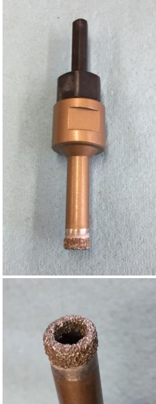
Fig. A-71(a) Diamond studded drill ( \text{Ø } \frac{1}{2} " DAMO). (b) Drilling into a concrete block using a drill press, process carried out over a plastic tray.
