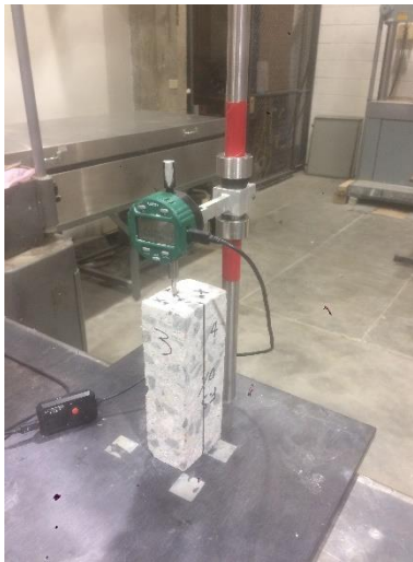
Figure 29 The method for measuring the change in length of sample under freezing process
