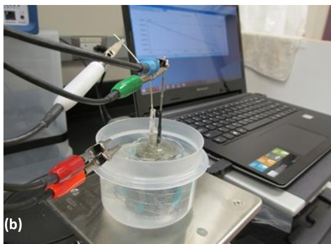
Figure C-1 (a) Schematic of the type-A consisting of concrete cast cylinder with embedded rebar steel, and provision for inserting a reference electrode. (b) Three-electrode EIS testing configuration. Pt-wire as counter electrode was spiraled around the concrete cylinder.
