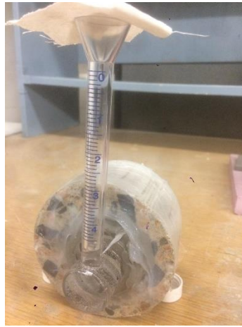
Figure 44 The sample is under the RILEM Tube Testing
