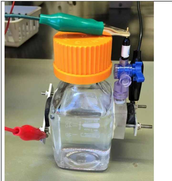
Fig. A-34 Experimental setup used for electrochemical testing.
