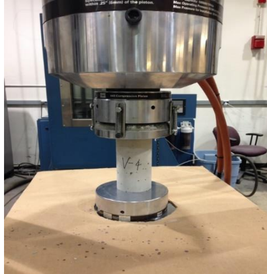
Figure 7 the sample under compression test
