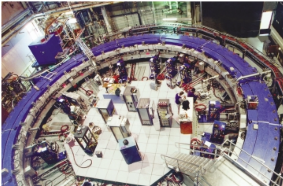
Figure 2.18. A crack in the Standard Model? The superconducting storage ring at Brookhaven is currently being used to measure the muon anomalous magnetic moment, g - 2 , to a precision of better than 1 ppm. Comparing experiment to theory provides a sensitive test of the Standard Model and proposed extensions. In fact, a recently published experimental result differed significantly from theory, prompting a reevaluation of the underlying theory and the discovery of an error. With 80% of the data yet to be analyzed, the physics community is watching this situation closely. Photo courtesy of Ripp Bowman.
