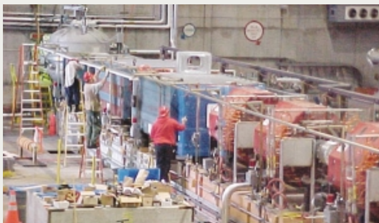
E158 at Stanford. The photograph shows the liquid hydrogen target chamber and the giant dipole and quadrupole magnets of the E158 forward-angle spectrometer under construction at SLAC. E158 is designed to measure the tiny weak force between two electrons to search for clues to a new “superweak” force.
