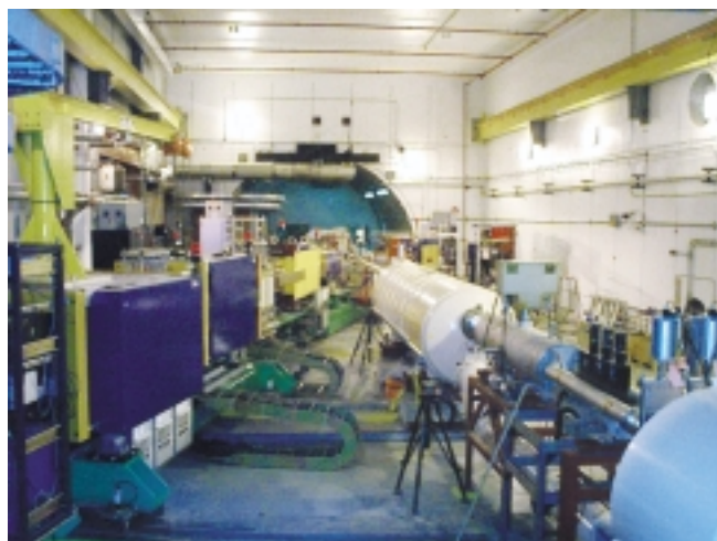
Figure 3.5. Detectors at RHIC. RHIC is currently instrumented with four detectors, two major ones (STAR and PHENIX) and two smaller ones (BRAHMS and PHOBOS). STAR, on the left, is a large-acceptance detector built around a central time-projection chamber (TPC) in a solenoidal magnetic field. Inside the TPC is a silicon vertex tracker for detecting secondary vertices. One of the smaller detectors, BRAHMS, is shown on the right; it specializes in measuring the fragmentation region of the collisions. Not shown are the PHENIX detector, which is composed of four spectrometers optimized for detecting and identifying electrons, muons, photons, and hadrons, and PHOBOS, the second of the smaller detectors, which is optimized for large event rates.
