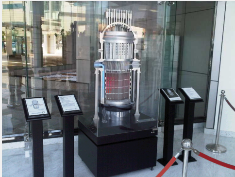
Scale Model of APR 1400 Reactor Pressure Vessel
