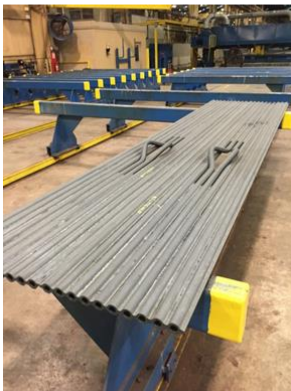
Figure 4-b HR6W prototype panels after the post-bend heat treatment
