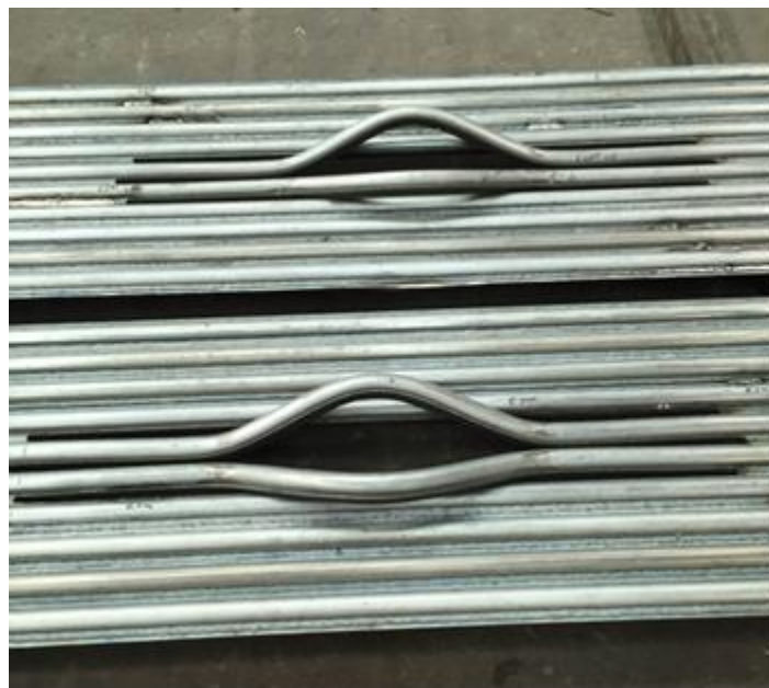
Figure 3-t Press openings in the HR6W panels
