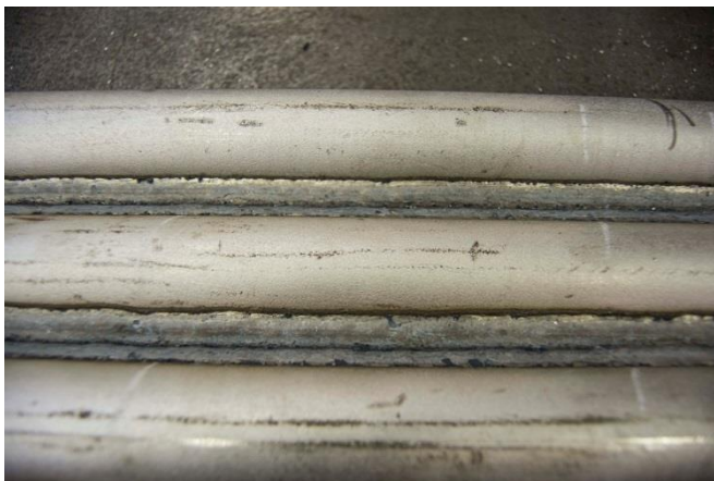
Figure 3-p Example of three-tube laboratory scale HR6W panels fabricated at the MTC
