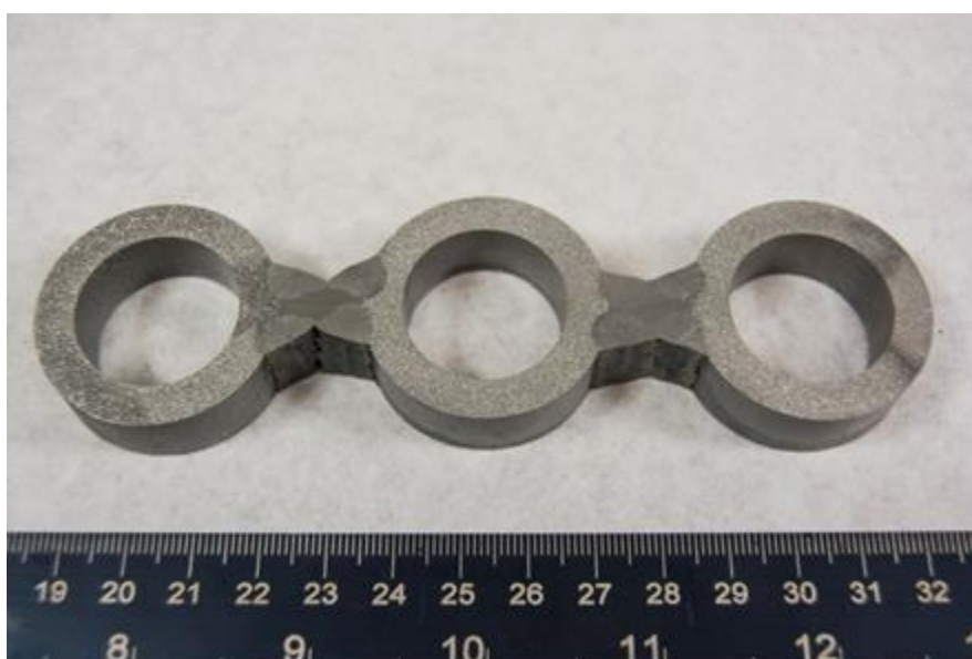
Figure 3-q Macrograph of three tube HR6W laboratory panel
