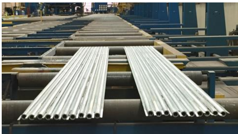
Figure 3-s Completed HR6W 10-tube shop sub-panels
