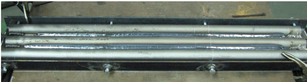
Figure 3-c Example of three-tube laboratory scale panel fabricated at the MTC
