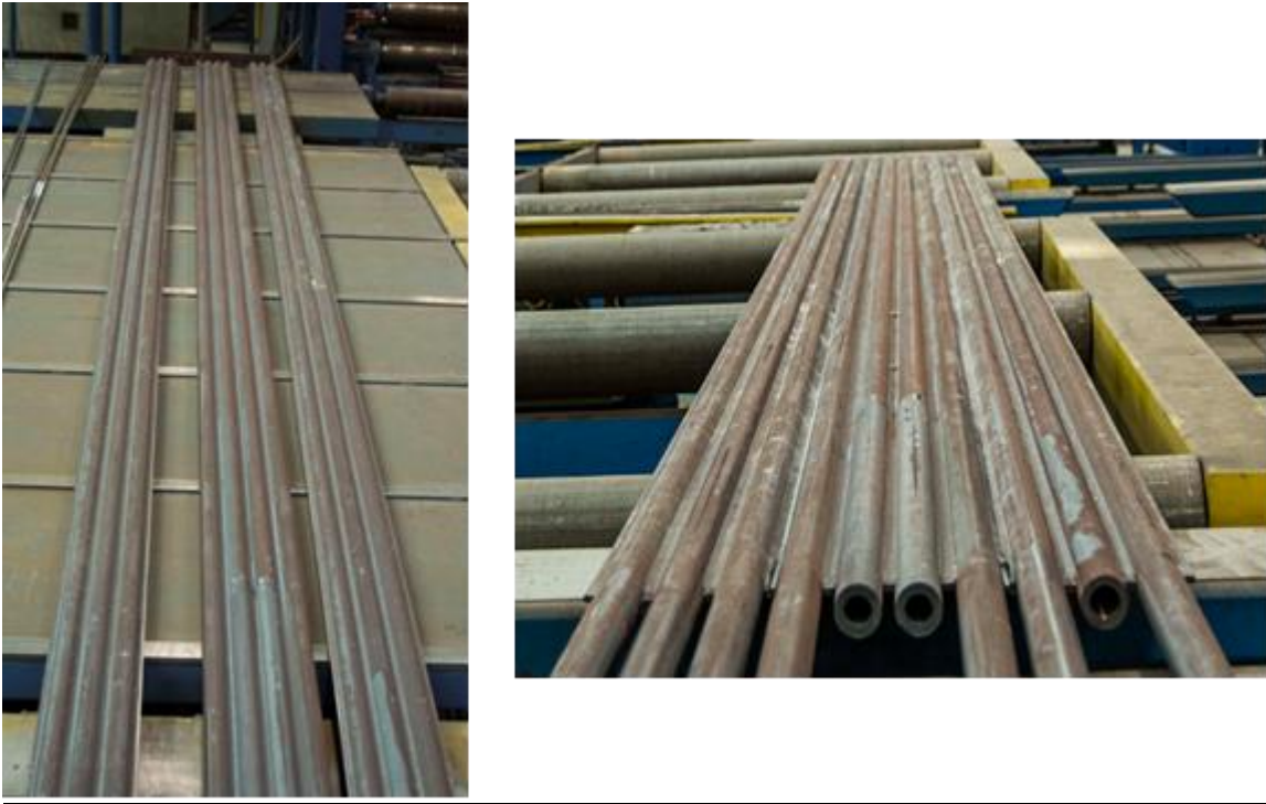
Figure 3-i Completed sub-panels prior to final assembly (left) and completed 10-tube panel (right)
