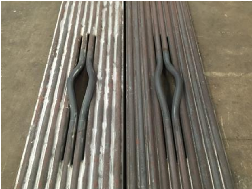
Figure 3-l Photograph of the press openings in T92 sub-panels
