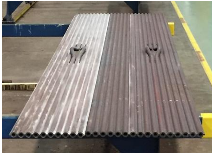
Figure 4-a Completed 26-tube Grade 92 membrane panel
