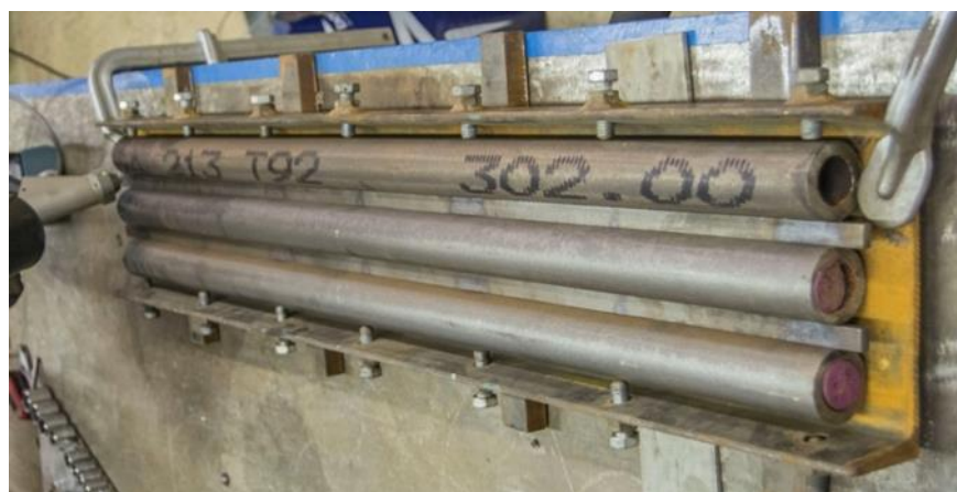
Figure 3-a Lab Scale T92 Panel Ready for Welding
