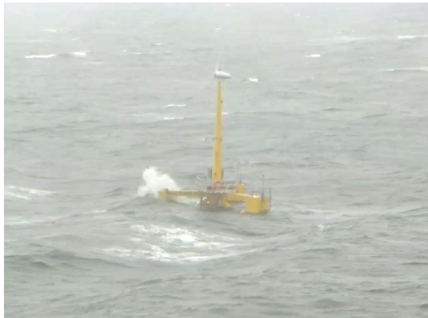
Figure 33 VoltturnUS 1:8 subjected to scaled extreme 50-year design conditions of ABS DLC 1.6 on November 1 st , 2013
