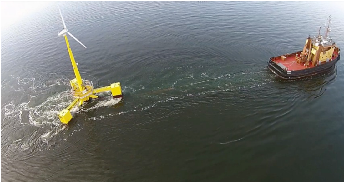
Figure 37 VoltturnUS 1:8 Recovery Tow Configuration
