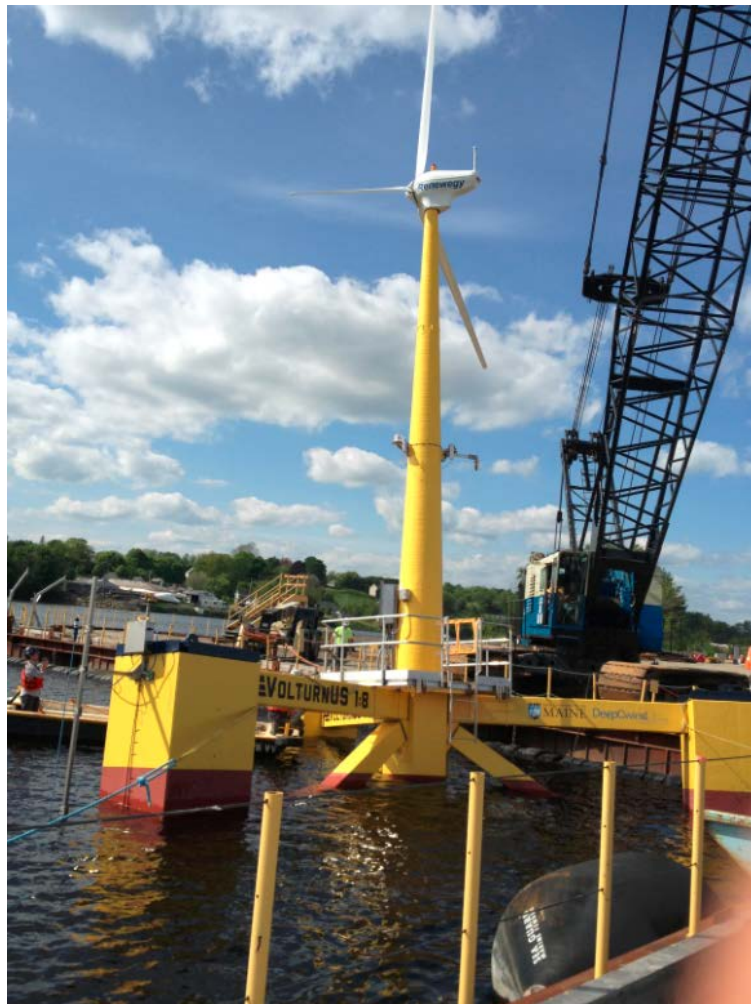
Figure 28 Incline Testing Dockside
