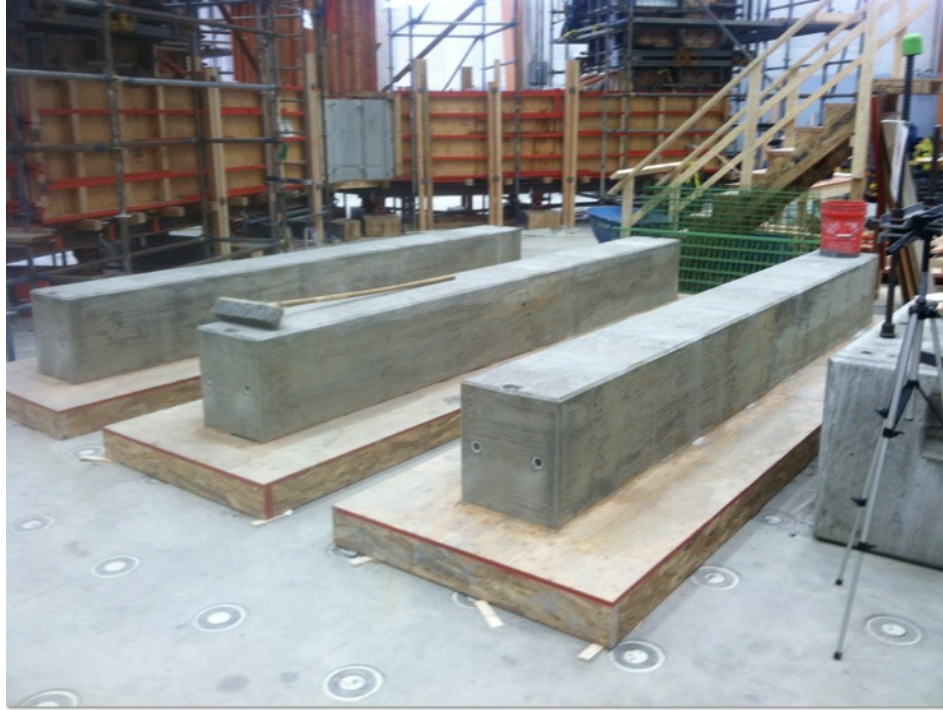
Figure 17 Compression Struts Cast Separately
