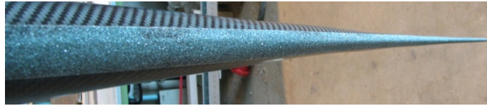
Figure 21: Image of roughened leading edge of model wind turbine blade.
