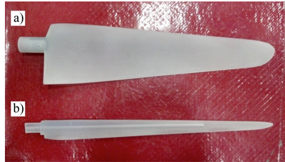
Figure 127: Images of a) redesigned, thrust-matched blade and b) original geometrically-scaled, NREL 5 MW reference wind turbine blade.
