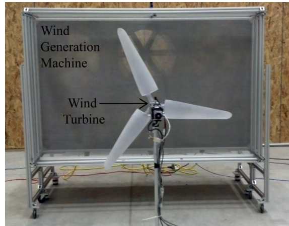
Figure 132: Image of the test wind turbine being tested behind the wind generation machine.
