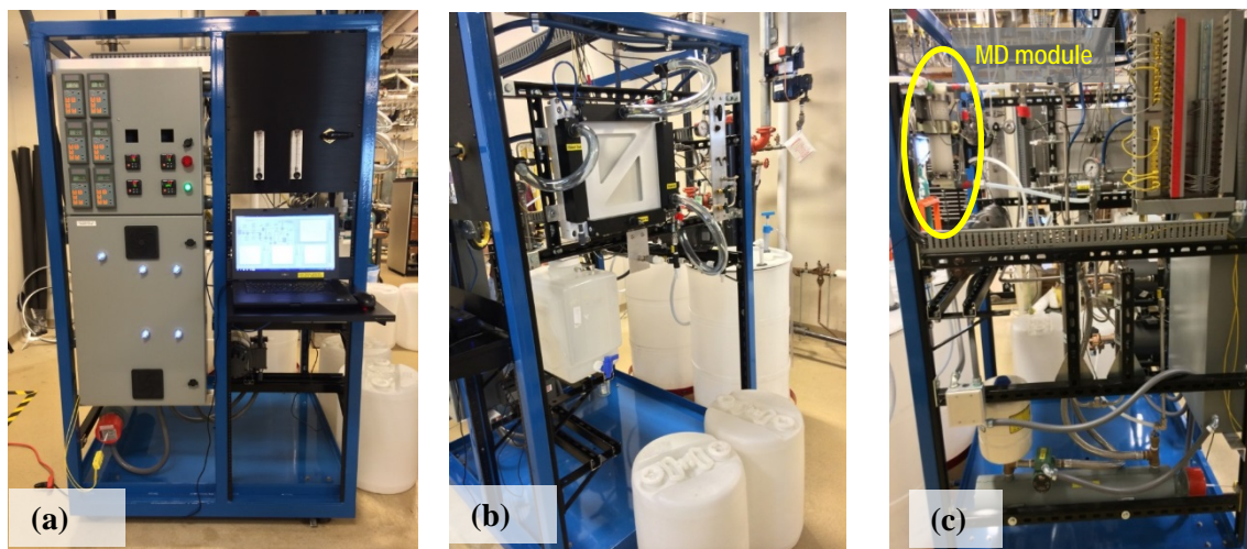
Figure 4-54. Photos of bench, integrated FO-MD system: (a) front view, (b) right-side view, and (c) left-side view with M-HF200 MD membrane module (area \sim 0.64 \text{ m}^2 ) highlighted.
