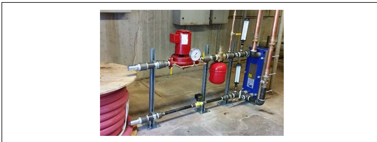
Figure 3-19. Secondary cooling-water loop set up at the test site to support field-testing of integrated FO-MD prototype
