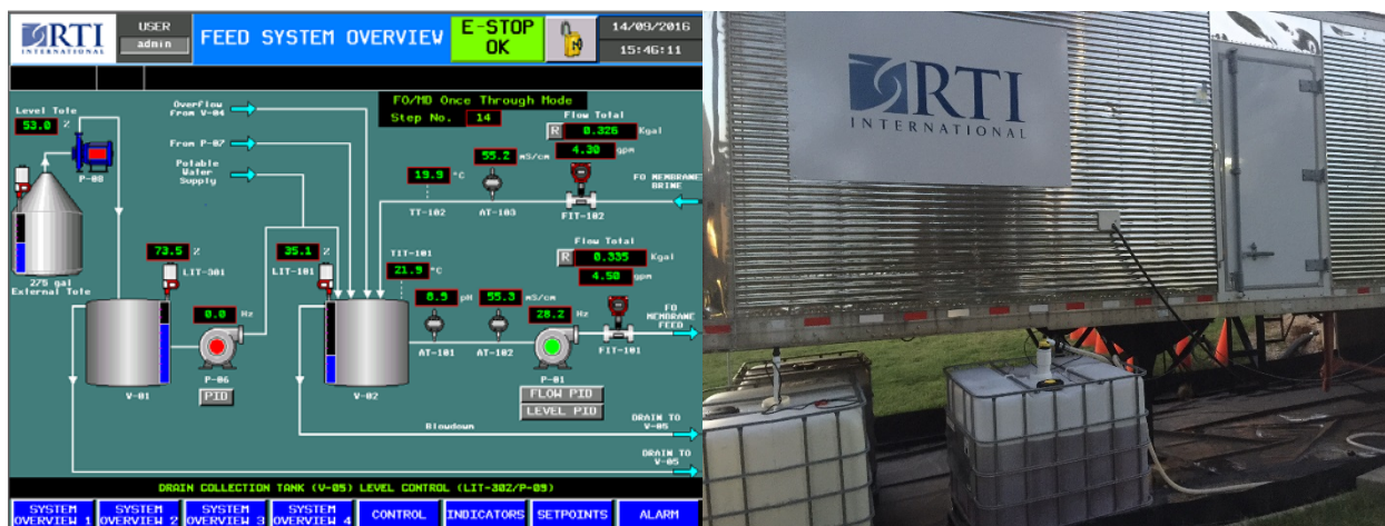
Figure 3-23 HMI interface and photograph of Feed System of the FO-MD prototype in operation.
