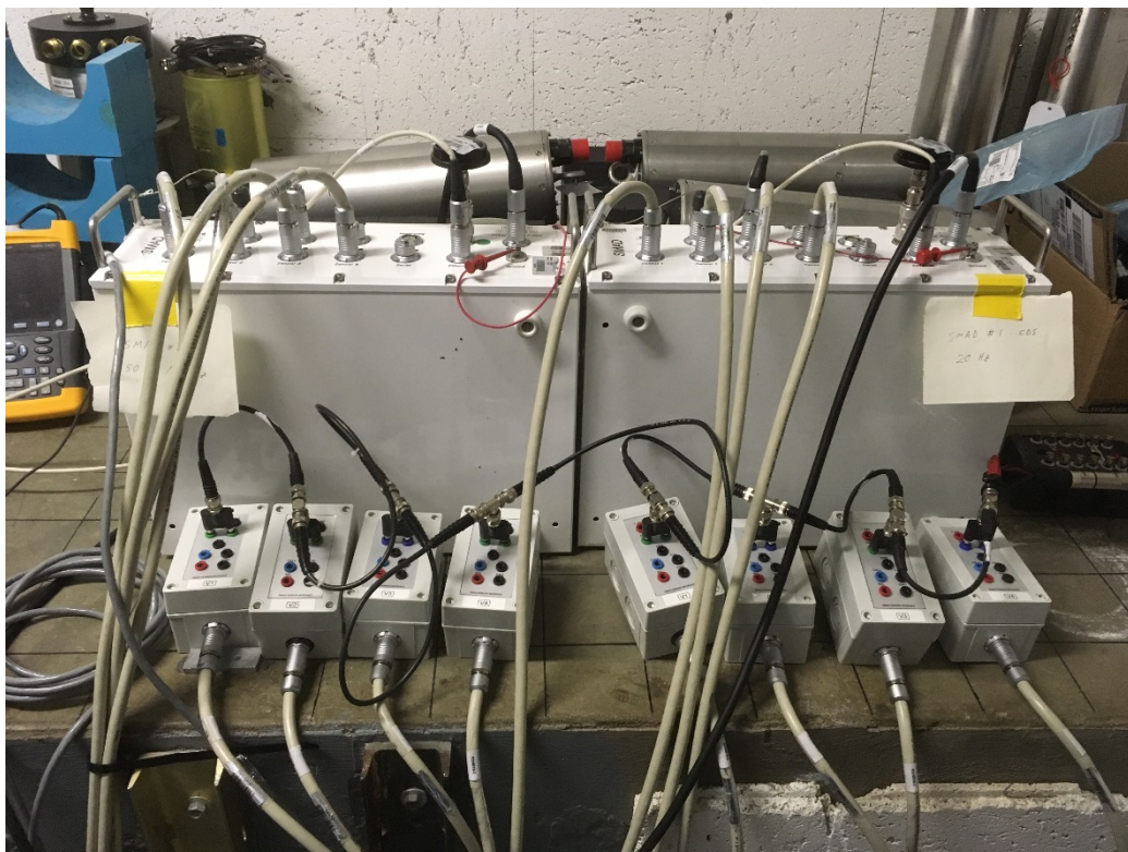
Figure 3 SMAD Digitizers within FACT Bunker
