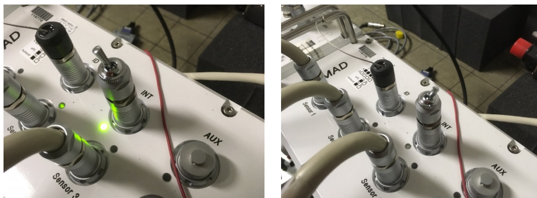
Figure 100 SMAD Digitizer Case Open Switch
