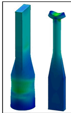
Figure 26. Stress analysis of design modification of the pin and cap fastener
