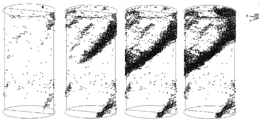
Figure62. Damage events during uniaxial compression (step= 175,185, 190, 200).
