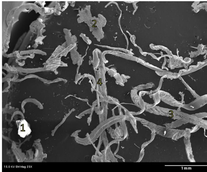
Figure 20: Image of foreign material debris within the heater inlet at 504.
