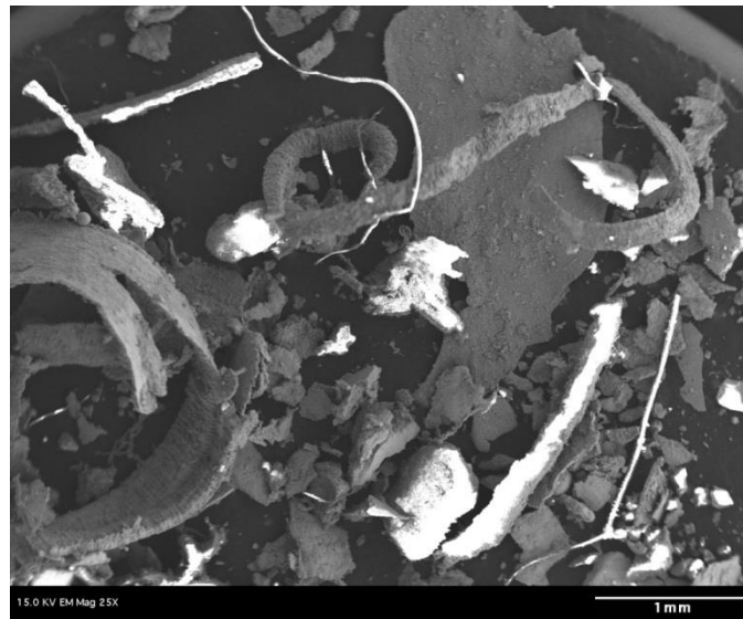
Figure 14: SEM image of foreign material from the expansion tanks.
