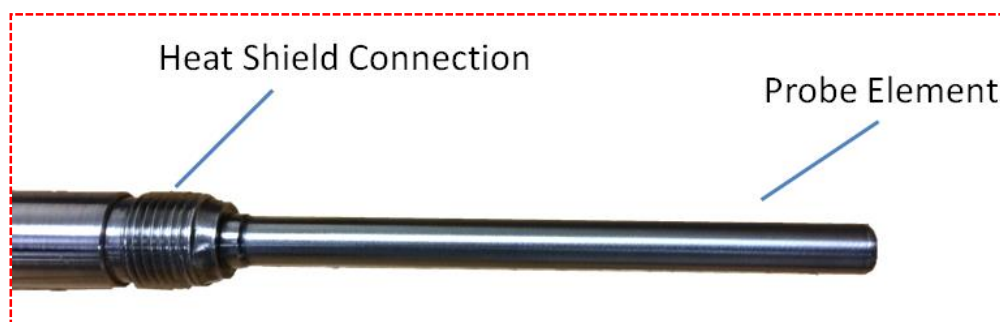
Figure 29: Photo of 316L ER device with heat shield removed. Reference element internal to the device.
