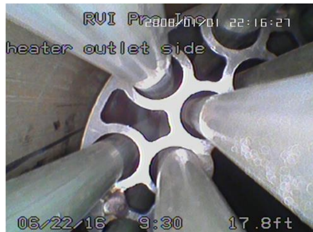
Figure 19: Interior photos of the inlet and outlet areas of the heaters.
