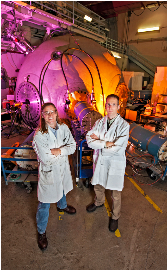
Researchers prepare to conduct an experiment in the spherical firing tank, the largest chamber located at HEAF, capable of detonating 10 kilograms (22 pounds) of explosives.
