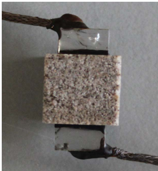
Figure 1. The \text{LiNbO}_3 transducers attached to opposing faces of the 9.13 x 6.65 x 8.32 mm Berea sandstone sample using high temperature epoxy
