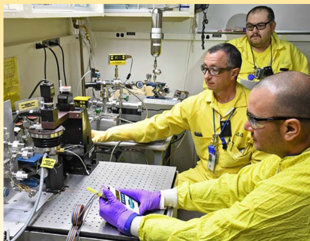
MST-16 technicians (from front) Jesse Salazar, Richard Salazar, and Ernesto Gallegos monitor gas sampling equipment used in support of the pit surveillance and life extension programs.
