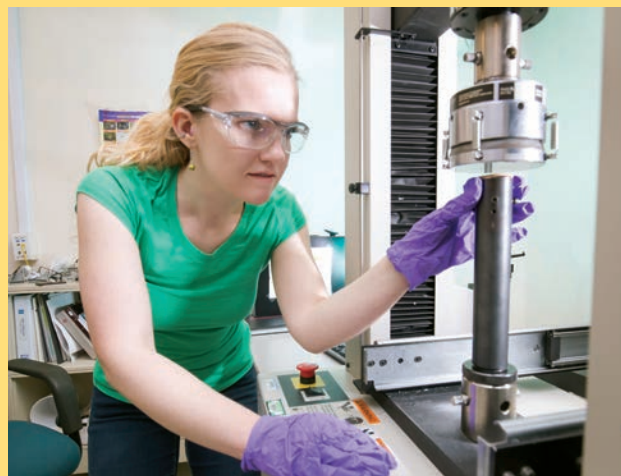
MST-7 technologist Stephanie Edwards uses a load frame to test the stress/strain properties of a silicone foam.
