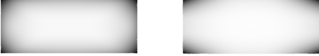
Figure 5: The left image is the COMSOL simulation of the rectangular wire problem. The analytic solution is shown on the right, and represents the formula derived in the box above. The current density on the bottom center and top center is too large in comparison to the analytic solution. The current on the center of the vertical sides is also too large.
