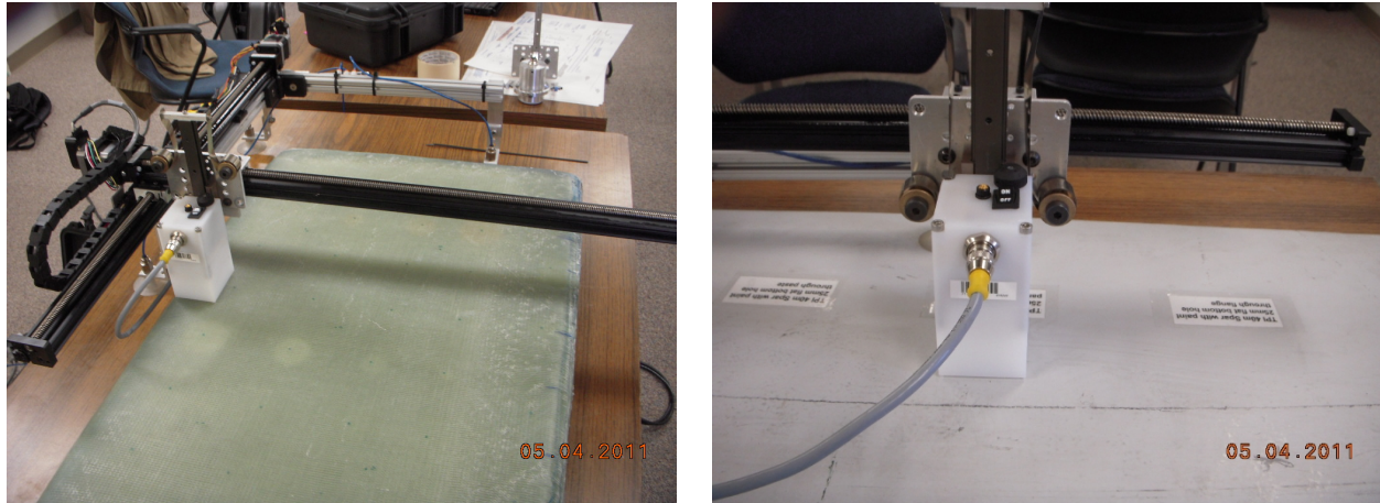
Figure 6-104: Evisive Microwave Inspection System with 10 GHz Probe
