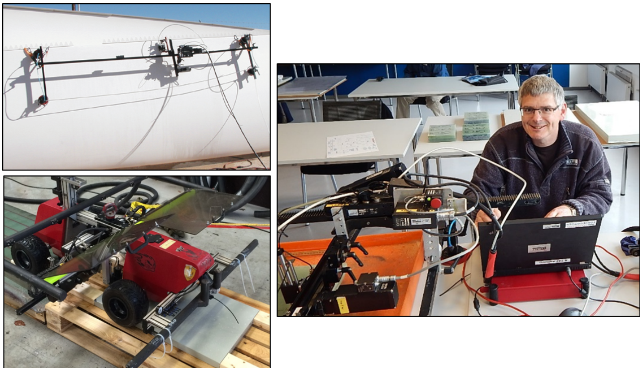
Figure 6-33: Force Technology P-Scan UT System with ATS-1 Automated Track Scanner and AMS-46 Tractor Scanner
