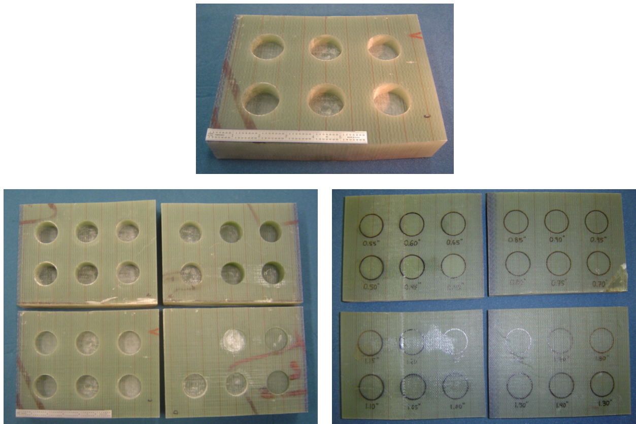
Figure 3-12: Laminate Thickness NDI Feedback Specimens Made From a Retired Blade – Flat Bottom Holes Placed in Representative Laminate Section to Simulate Delaminations and Backside Disbonds
