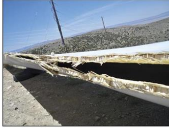
Trailing Edge Disbond and Fracture Damage
