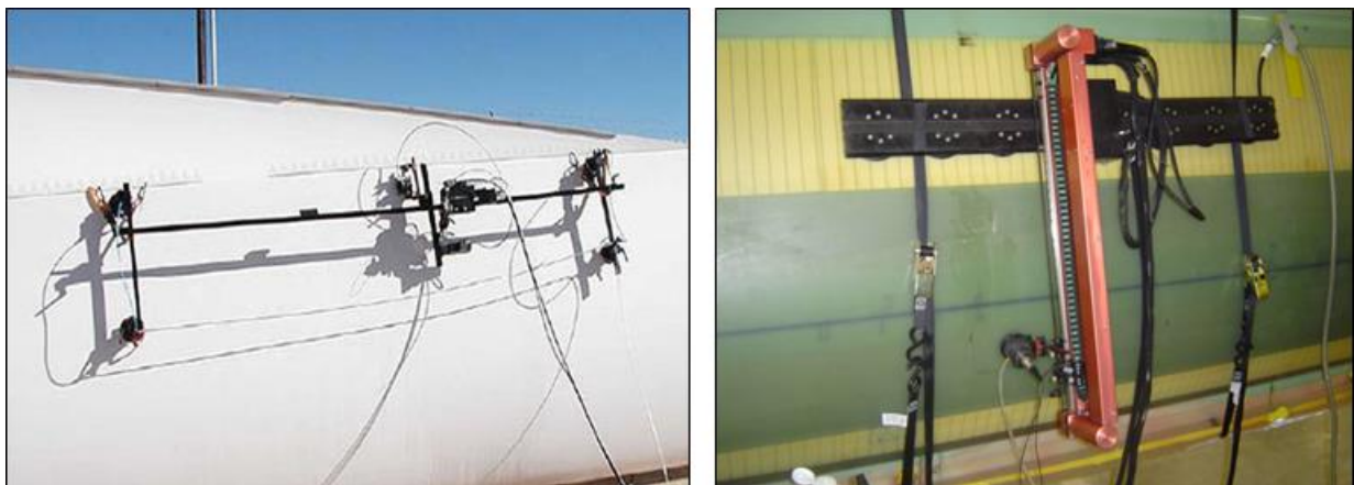
Figure 2-15: Unmanned Aerial Systems and Ground-Based Devices Used to Conduct Visual Inspection of Wind Blades
