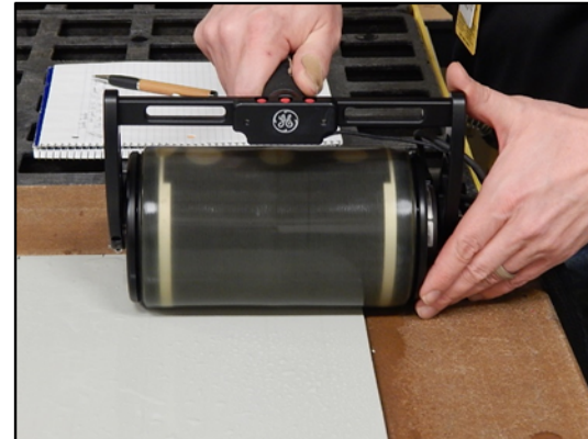
1 MHz GE RotoArray (1 MHz, 64 Elements)
