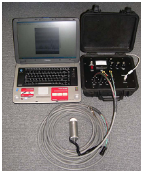
Figure 5-68: Basic Equipment Set-up for Microwave Inspection
