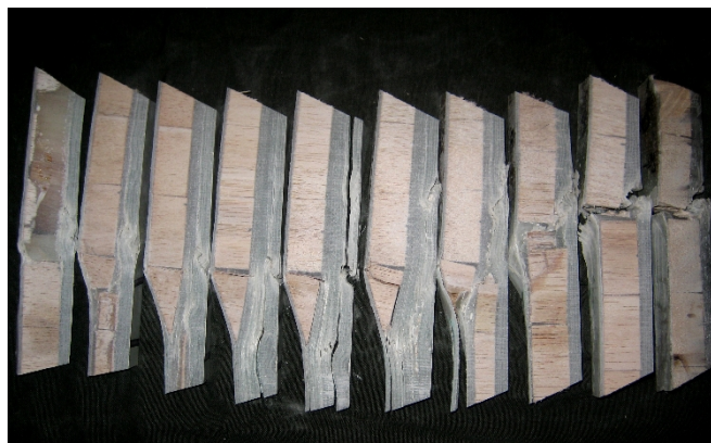
Figure 2-4: Figure Comparing Pristine Blades with Cracks, Delaminations and Other Laminate Fractures that Can Occur in Wind Blades
