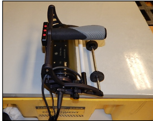
GE RotoArray (500KHz, 60 Elements)
