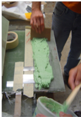
Template for flaw insertion
