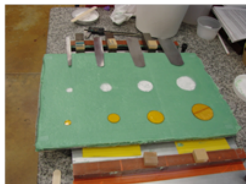
Final look before top laminate is put in place
