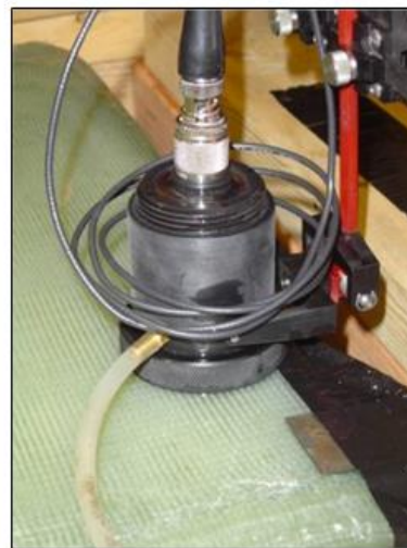
Figure 5-41: Variation on Water Column Shoe that Includes a Threaded Housing to Allow for Adjusting the Length of the Water Path or Column Height (Patent Pending)
