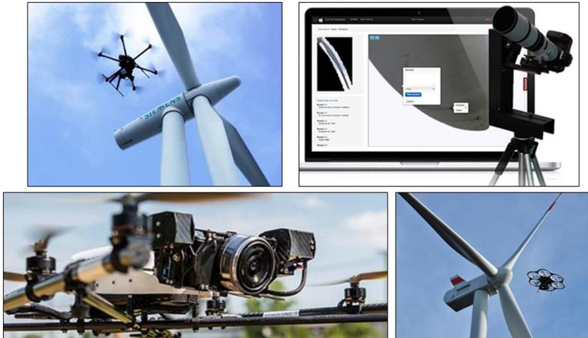
Figure 2-15: Unmanned Aerial Systems and Ground-Based Devices Used to Conduct Visual Inspection of Wind Blades
