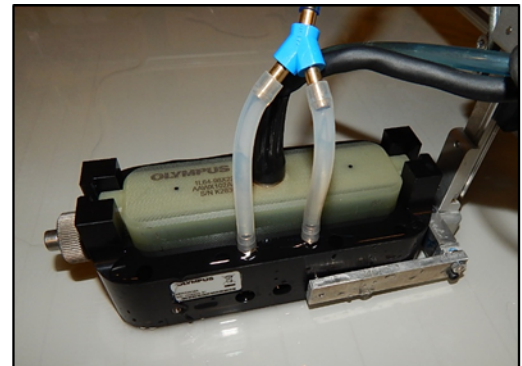
Figure 6-30: Sample Deployment of Advanced NDI Equipment - Phased Array Ultrasonics and the P-Scan Single Element UT Scanning System
