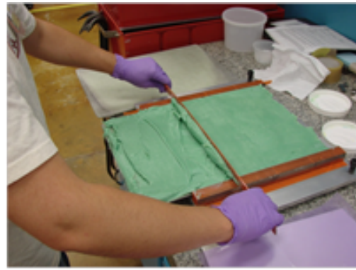
Screeding of adhesive to specific thickness
