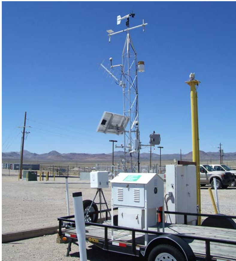
Figure 1-4. TTR Station 400 measures radiological and meteorological conditions near the ROC
