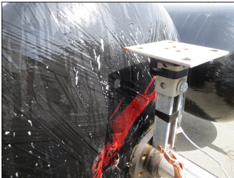
Figure 67 - Snoop bubble formation, Titan #2 (rear) after Transfer 6
