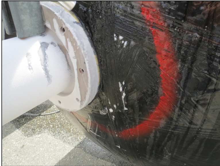
Figure 64 – Snoop Bubbles at Titan #2, after Transfer 6
