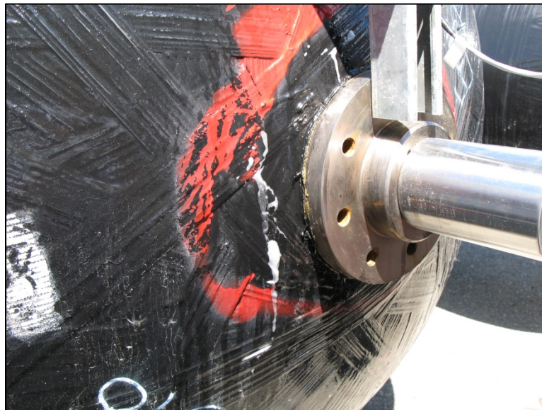
Figure 31 – Snoop bubbles after transfer (Titan #2)
