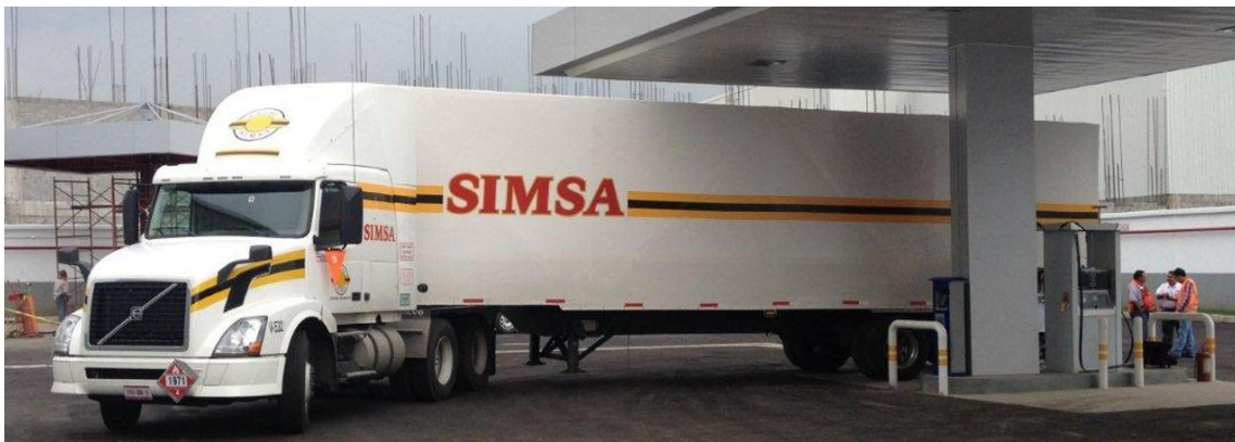
Figure 17 - The Hexagon Composites TITAN® Magnum Trailer System [GVW = 42 500 kg (3 axles)]
