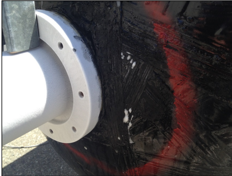
Figure 48 – Snoop bubble formation on Titan #2 (front)
