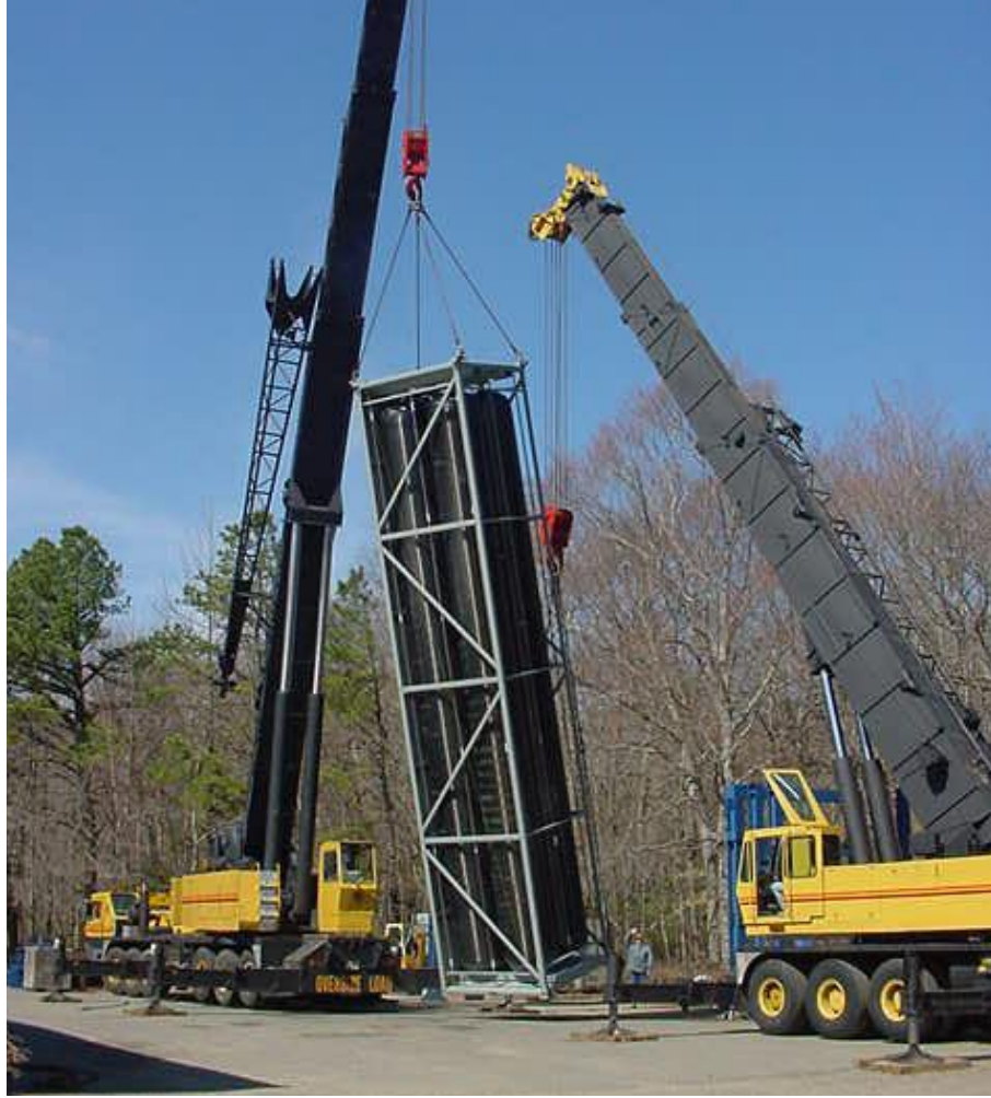
Figure 3 – ISO 1496 testing of TITAN® container (longitudinal inertia test).
