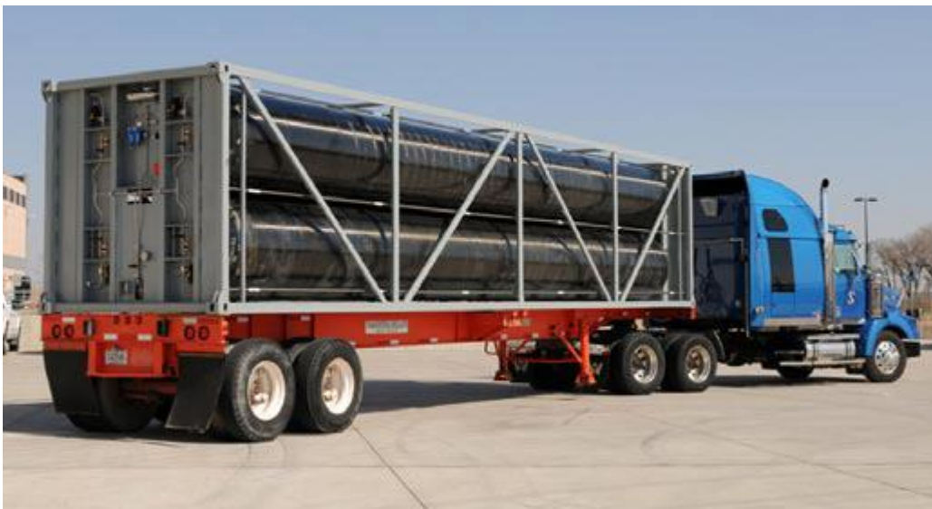
Figure 2 - TITAN® container structural and bonfire test unit.
