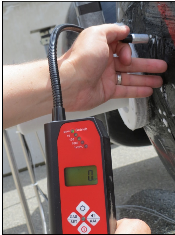
Figure 66 – Handheld detector, Titan #2 (0 ppm, 1-2 cm from bubbles)
