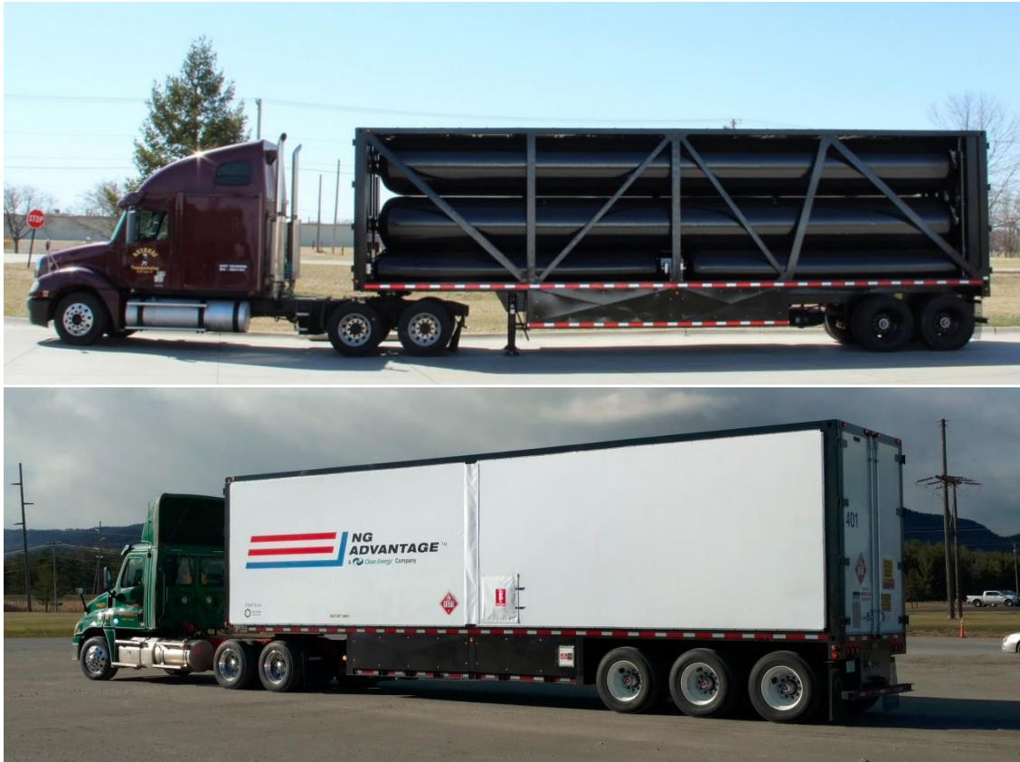
Figure 18 - The Hexagon Composites TITAN® XL Trailer System [GVW = 42 500 kg (3 axles)].
