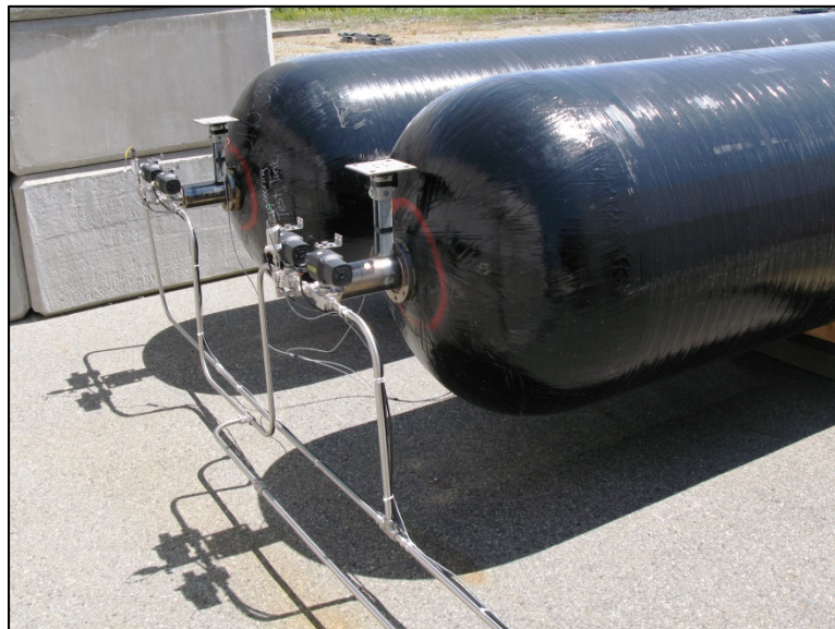
Figure 5 – Test Titans connected with Actuated Valves
