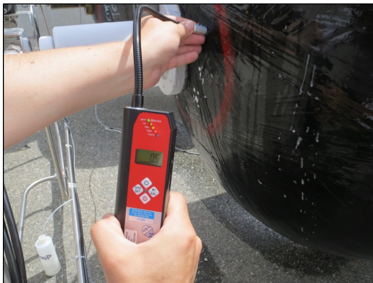
Figure 65 – Handheld detector, Titan #2 immediately after Transfer 6 (0.5 vol%)
