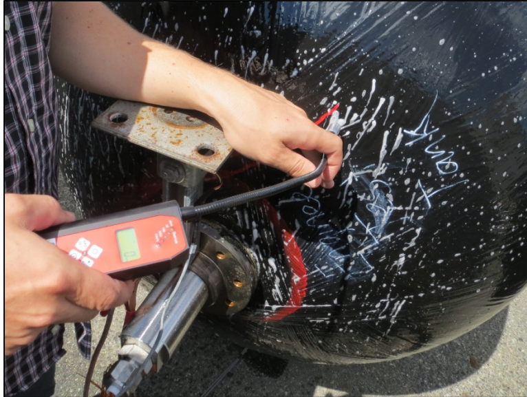
Figure 83 - Leak Check at Titan 2 (0 ppm at 1 cm from bubble location, rear)
