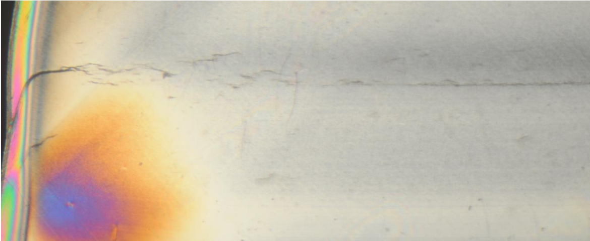
Figure 11 – Close up of injection molded HDPE (5.3 mm) after 2 hydrogen cycles
