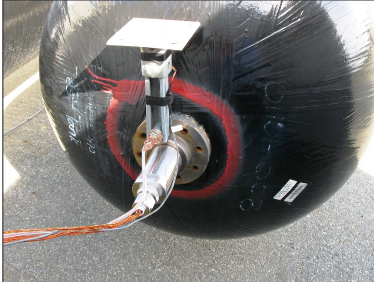
Figure 4 – End Fittings with Cameras installed in Titan #1
