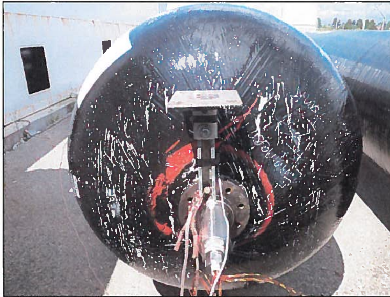
Figure 85 – Transfer 8, Snoop bubbles at rear of tank
