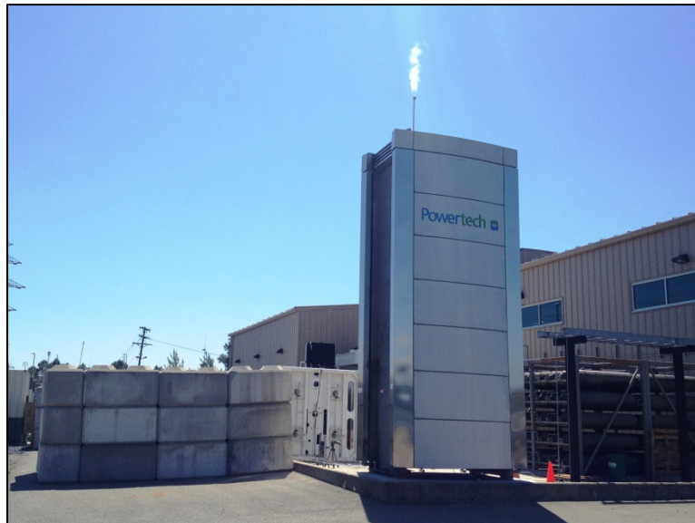
Figure 47 – Venting Titan #2 to 25 barg
