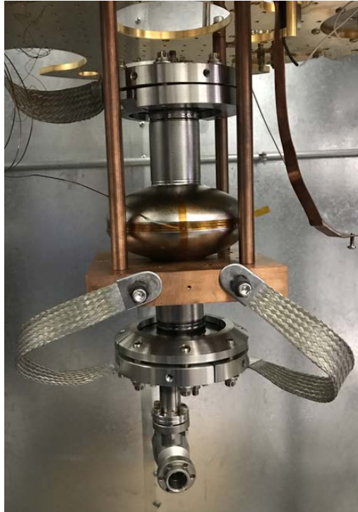
Figure 7. The Jefferson Lab 2.2 GHz SRF Cavity mounted onto the Mixing Chamber plate (Coldest surface) of the UMD Dilution Fridge.
