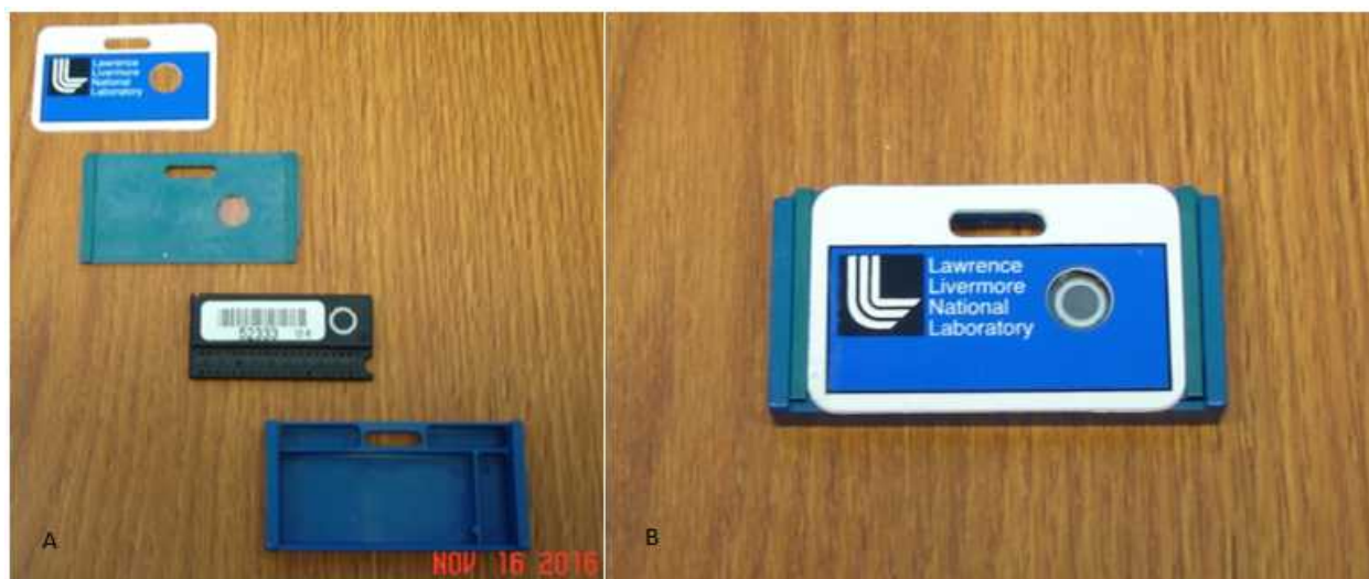
Figure 1. (A) Expanded view of contents of LLNL Dosimeter (B) Assembled LLNL Dosimeter
