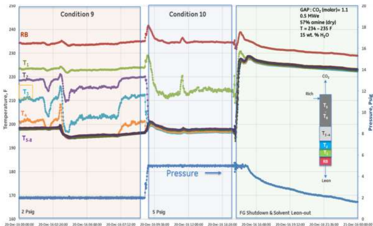
Figure 85. SSC campaign (Phase 2 – Pressure effect): SSC temperature profile
