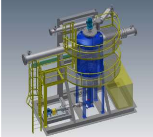
Figure 15. CSTR Design: Skid Structure (3D model, Chempro)
