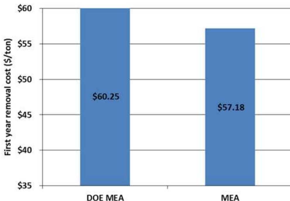
Figure 117. Comparison of first year removal cost of CO 2 using MEA vs. DOE estimated value 2
