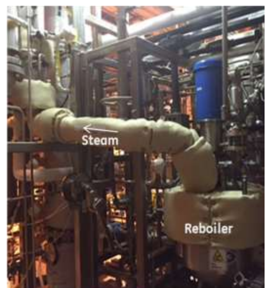
Figure 53. Steam Stripping: Bench scale system (2kW e ) installed at GE GRC
