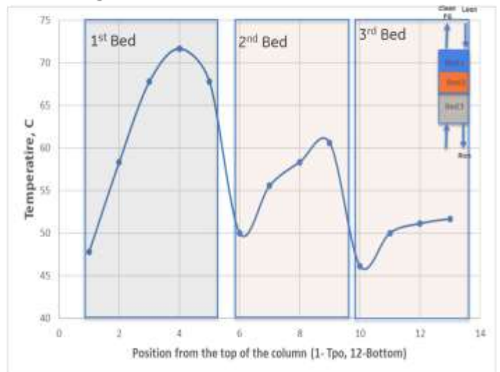
Figure 69. Absorber temperature profiles: Bench scale (2 kW, no inter-stage cooling) vs. Pilot Scale (0.25 MW e , 2 inter-stage cooling)
