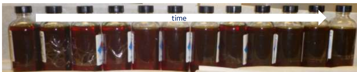
Figure 94. Solvent Degradation (SSC Campaign): Absorber samples = f (time) The dark amber initial color is indicating that the starting solvent of the SSC campaign had been slightly contaminated with used solvent from the CSTR campaign.
