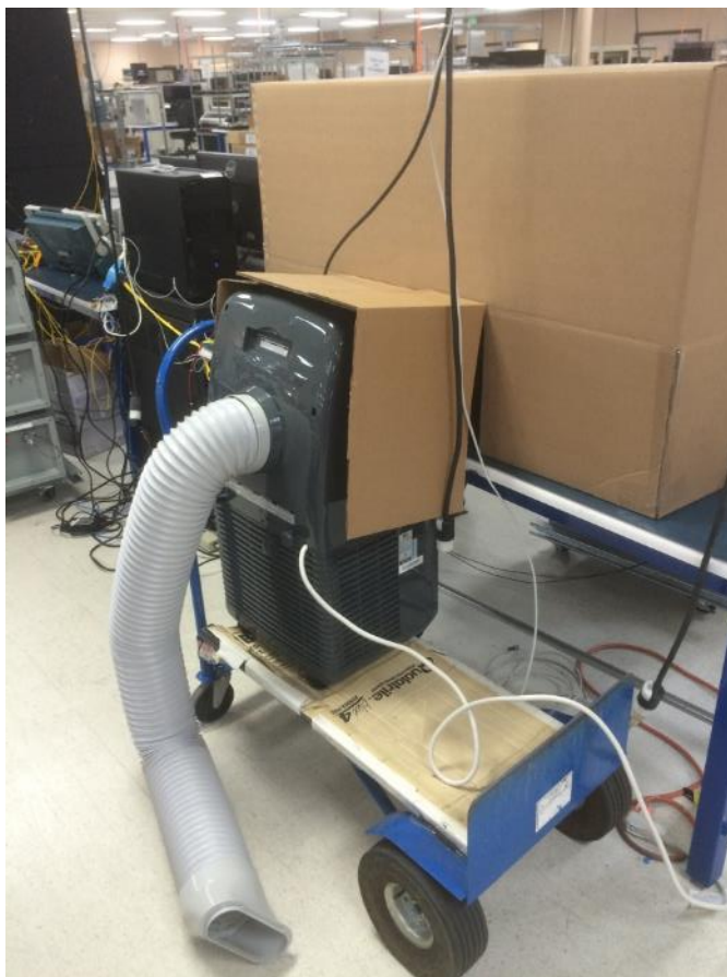
Figure 9 Temperature enclosure and cooling system
