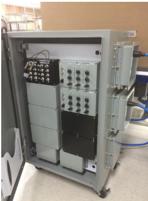
Figure 4 Production Test Station Interface to SHDAS DWR
