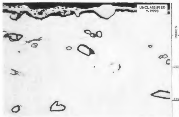
Fig. 3.2.13. Zirconium Specimen from Hot Leg of Inconel Thermal-Convection Loop Which Circulated Sodium for 1000 hr at a Hot-Leg Temperature of 1500^{\circ}\text{F} and a Cold-Leg Temperature of 1230^{\circ}\text{F} . As-polished. 1000X. Reduced 44%. (Secret with caption)
