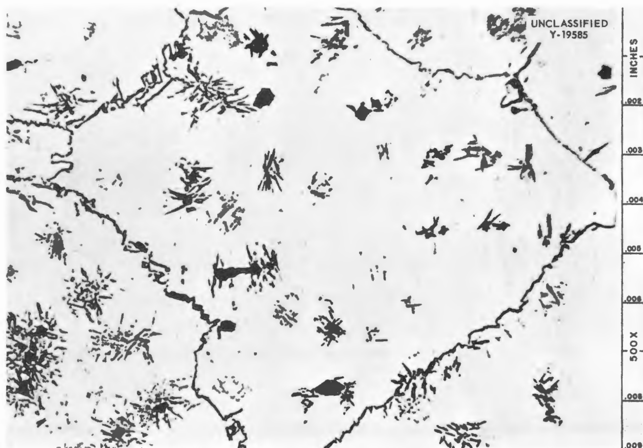
Fig. 3.3.12. Precipitate in Oxidized and Aged Niobium-Uranium Alloy. 500X. (Confidential with caption)
