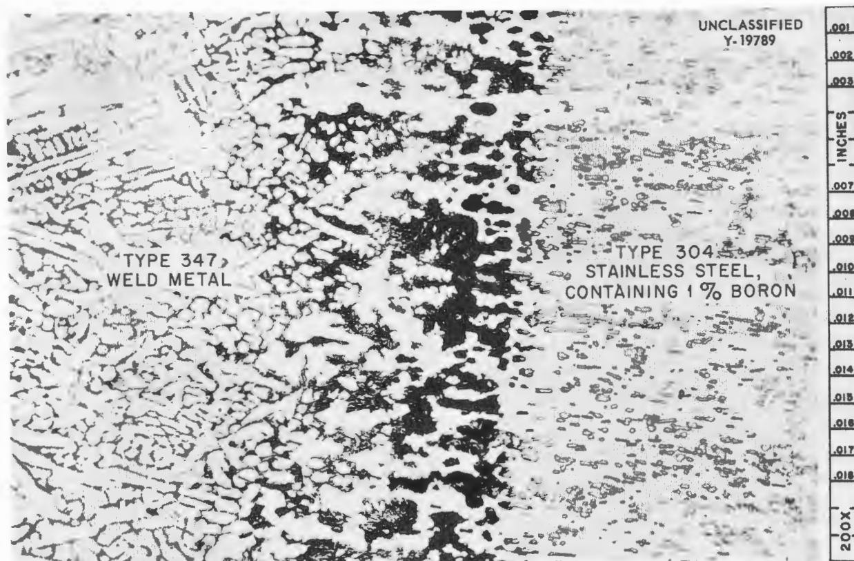
Fig. 3.4.24. Type 304 Stainless Steel Containing 1% Boron Inert-Arc Welded with Type 347 Stainless Steel Weld Metal. The complex borides visible as particles in the parent plate reacted with the type 304 stainless steel matrix and the weld metal to form a eutectic at the fusion line. 200X.
