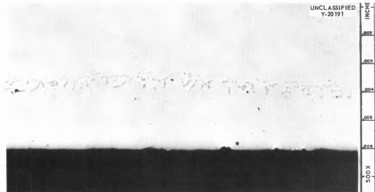
Fig. 3.4.13. Diffusion Layer Between Inconel Cladding and Copper Fin. As-polished. 500X.
