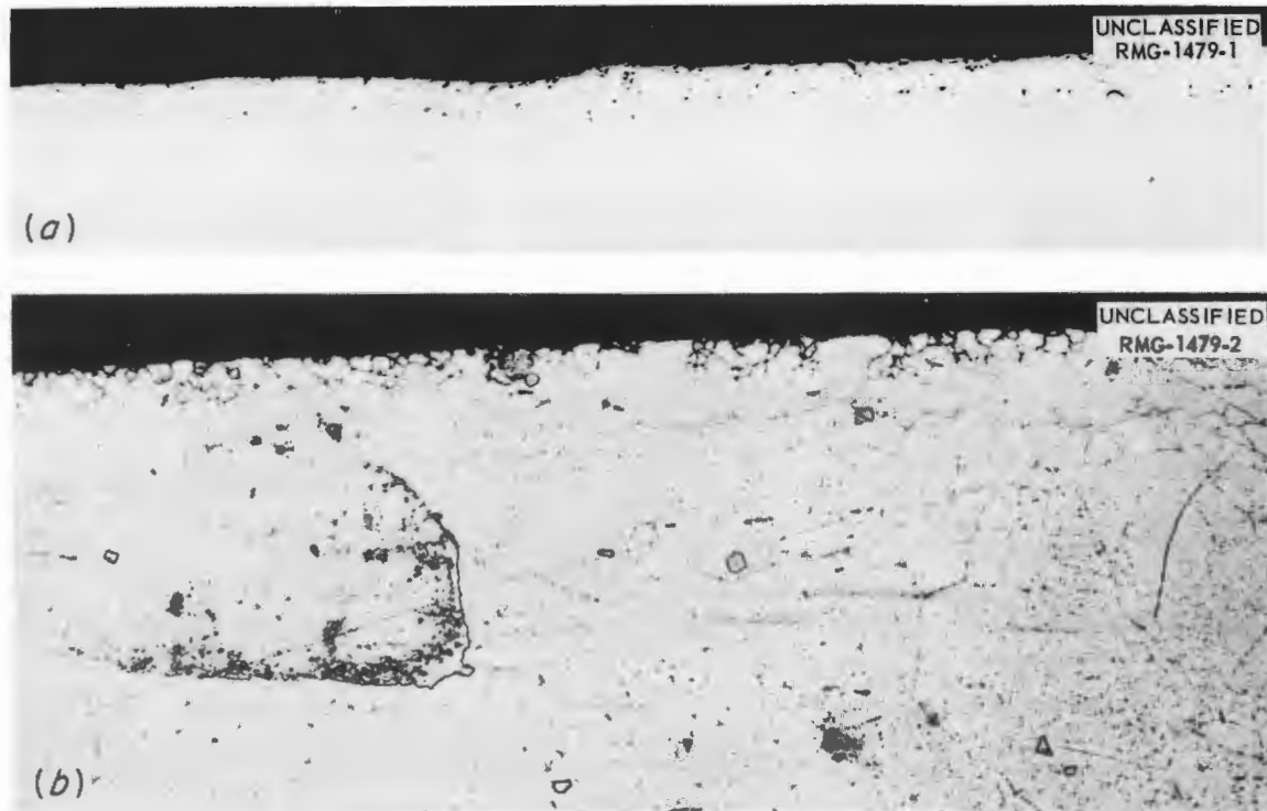
Fig. 4.2.17. Metallographic Sections of Irradiated Inconel Capsule No. 1. (a) Unetched. (b) Etched. 250X.
