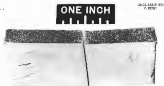
Fig. 3.4.26. Results of Guided-Bend Ductility Test of Type 304 Stainless Steel Containing 1% Boron. Specimen scratched to a depth of 0.020 in. before test.
