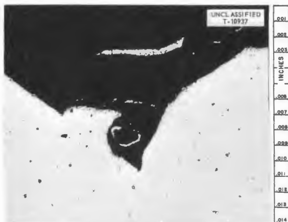
Fig. 3.7.5. Photomicrograph of Typical Tubing Flaw Detected by Radiography. 250X. Reduced 32%.
