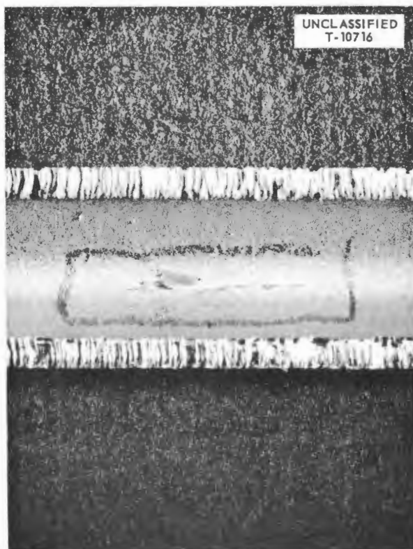
Fig. 3.7.6. Wide, Shallow, Gouge-Type Defect on Inner Surface of Tubing. This defect was detected by radiography. 8X. Reduced 7.5%.
