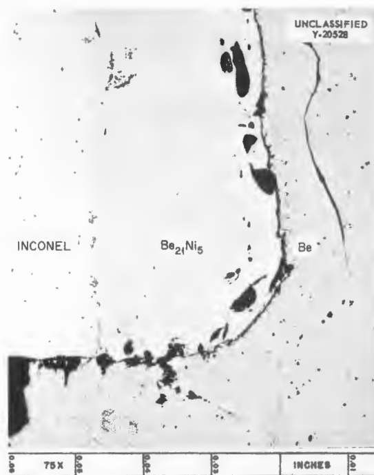
Fig. 3.2.12. Enlarged View of Area A of Fig. 3.2.11. Note alloying ( \text{Be}_{21}\text{Ni}_5 ) between Inconel sleeve and beryllium wall. Unetched. 75X. Reduced 29%. (Secret with caption)
