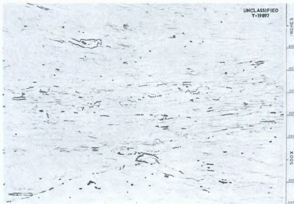
Fig. 3.3.10. An 80% Nb-20% U Alloy as Hot-Rolled at 1050°C. 500X. Reduced 2%. (Confidential with caption)
