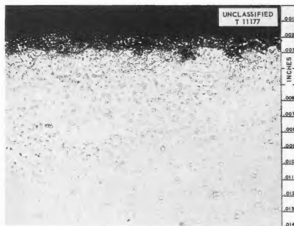
Fig. 3.1.4. Hot-Leg Attack in Hastelloy B Forced-Circulation Loop Operated with Sodium for 1000 hr at 1500° F. 250X. Reduced 32%.
