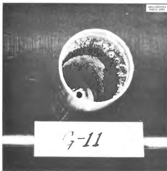
Fig. 2.2.7. Nickel Mass-Transferred Crystals on Nickel Container That Was Exposed to NaF- ZrF 4 Containing Added NiF 2 for One Week at 800°C Under Continuous Helium Sparging. (Confidential with caption)
