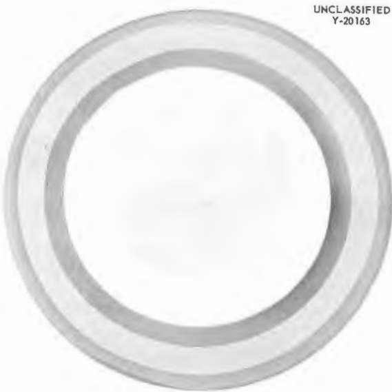
Fig. 3.3.7. Traverse Section of Three-Ply Control Rod Extrusion. 2.5X. Reduced 25%.
