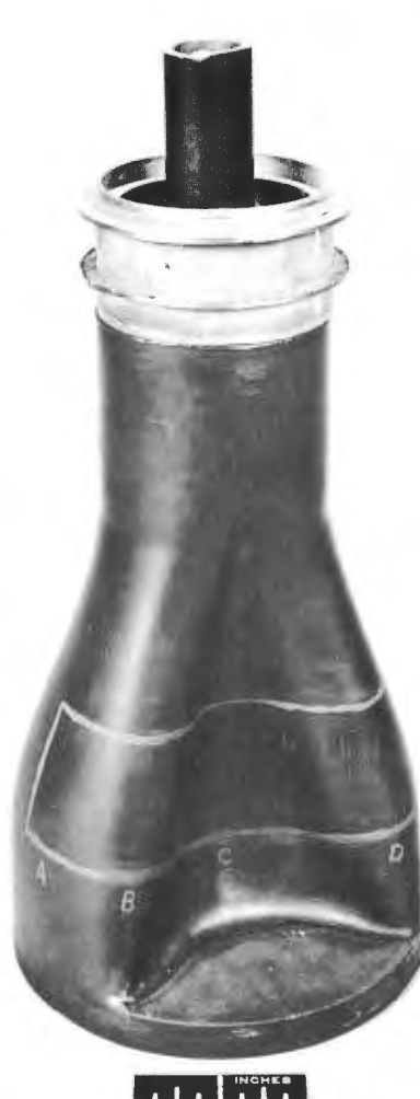
Fig. 1.1.2. The \frac{1}{4} -Scale Model of One-Half of Shell II After Creep-Buckling Collapse. —(Confidential with caption)
