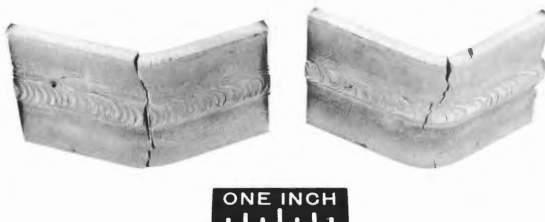
Fig. 3.4.23. Results of Guided-Bend Ductility Tests of Welded Type 304 Stainless Steel with 1% Boron Added. Weld metal, type 347 stainless steel. Bend radius, 2T .
