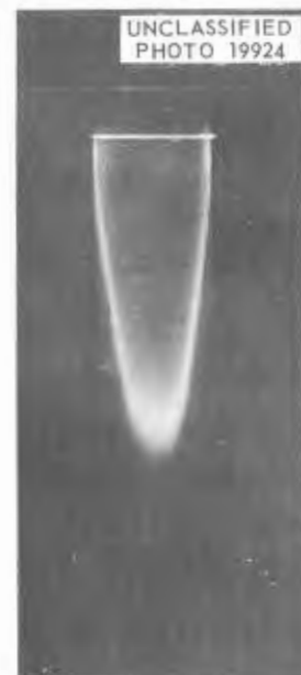
Fig. 4.1.7. Photograph of the Velocity Profile in a Circular Pipe Under Laminar-Flow Conditions.
