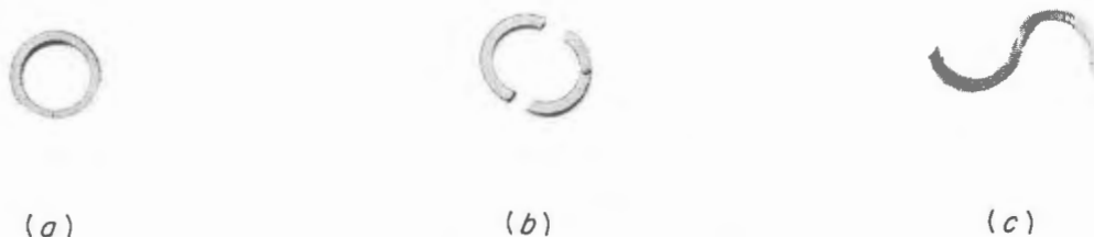
Fig. 3.4.8. Rings of Coast Metals Brazing Alloy No. 52 (a) As-Received, (b) As-Received and Fractured, and (c) Manually Deformed After Heating at a 100°F/hr Rate of Temperature Rise.
