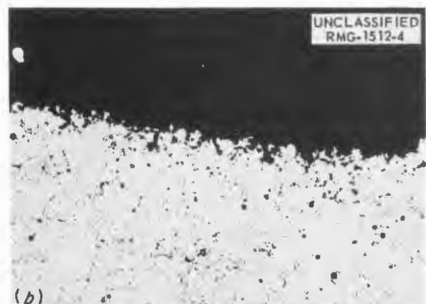
Fig. 4.2.10. Etched Structures of Specimens Shown in Fig. 4.2.9. (a) Specimen from loop No. 3. (b) Specimen from loop No. 4. 250X.
