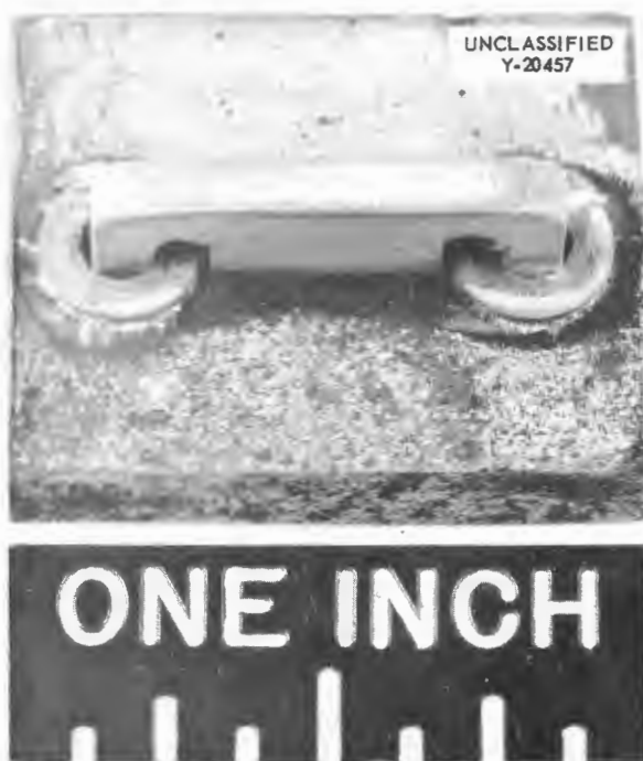
Fig. 3.2.10. Inconel Staple and Beryllium Block Assembly Following 1000 hr of Exposure to Sodium Thermally Cycled Between 500 and 1300°F Ten Times. (Secret with caption)
