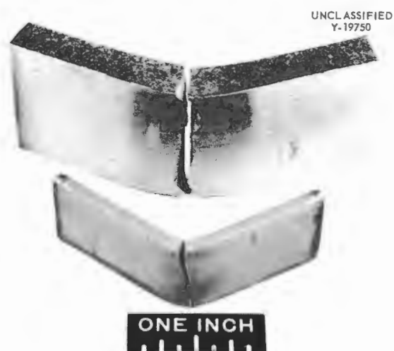
Fig. 3.4.25. Results of Guided-Bend Ductility Tests of Type 304 Stainless Steel Containing 1% Boron. Bend radius, 2T .
