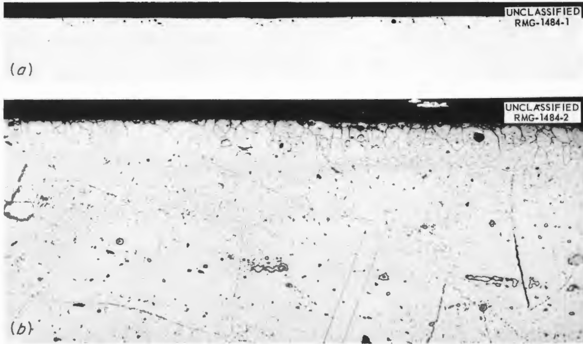
Fig. 4.2.21. Metallographic Sections of Unirradiated Inconel Capsule No. 5. (a) Unetched. (b) Etched. 250X.
