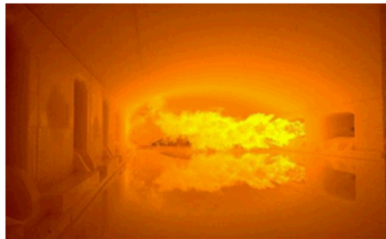
sooty flame in oxy-fuel glass melting furnace
