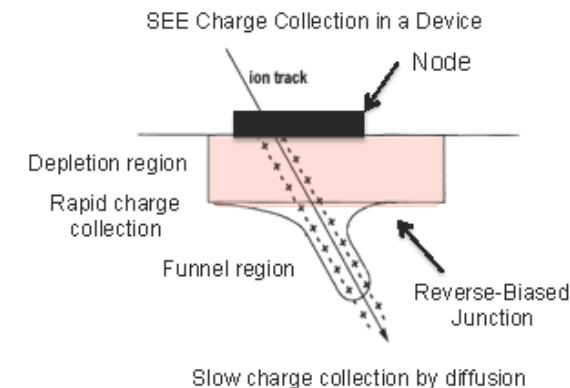
Nuclear reaction in semiconductor, leading to ionization
