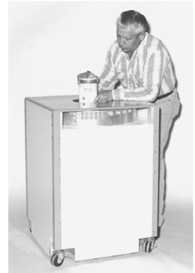
Plutonium Scrap Multiplicity Counter, used for accurate assays of plutonium metal, oxide, mixed oxide, or scrap (LANL PANDA Manual).
