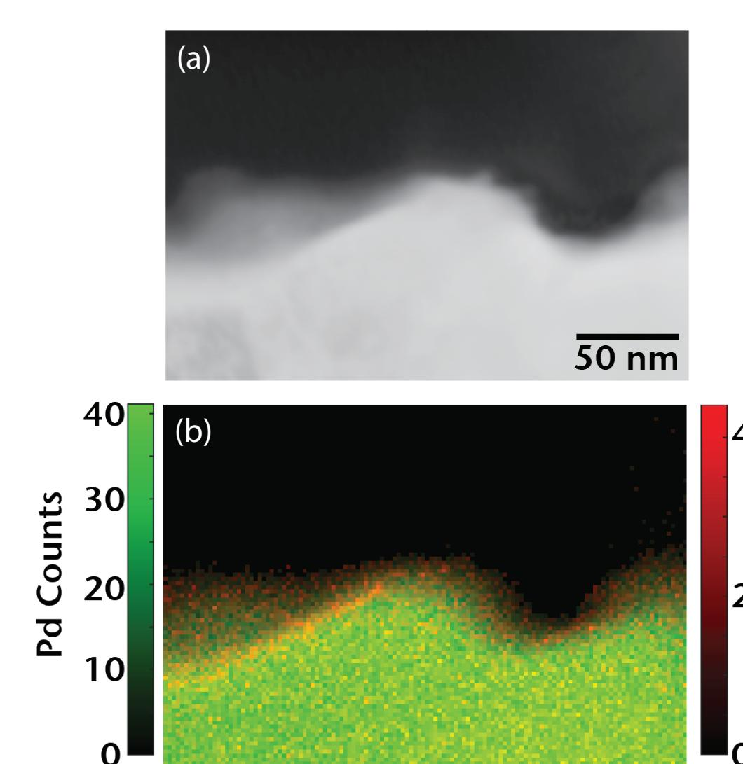
A second sample imaged at 30kV in the FIB/SEM using the STEM detector (HAADF) (a). EDS reveals a 5 nm Rh surface layer (b).
