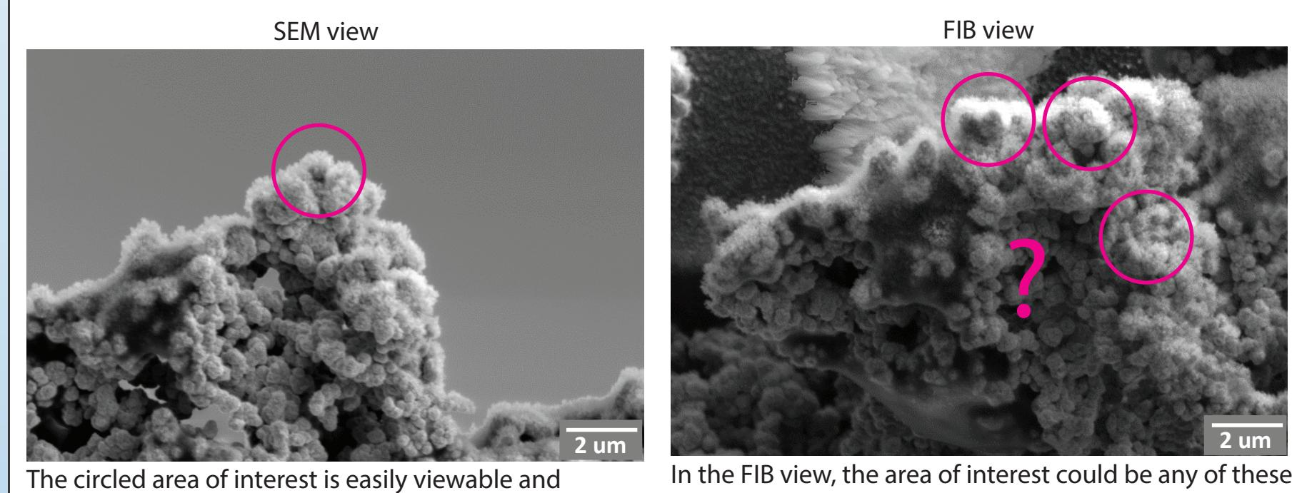
In the FIB view, the area of interest could be any of these locations, or could be out of view altogether.
