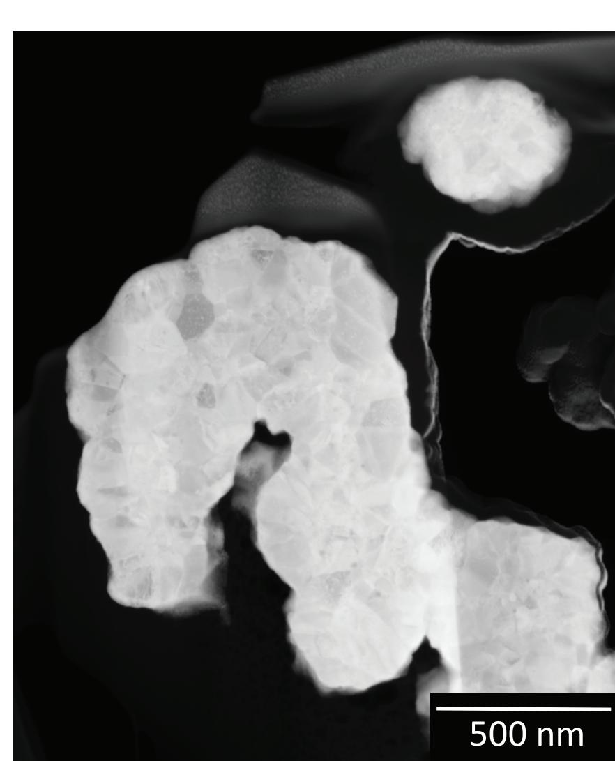
Here, the finished sample is being imaged at 30kV in the FIB/SEM using the STEM detector (HAADF).
