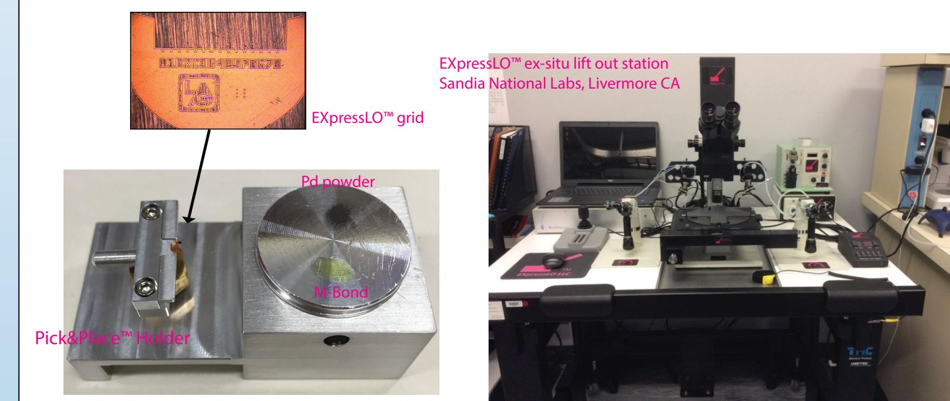
A small amount of powder was sprinkled onto one side of an Al stub. A small amount of M-Bond was placed on the other side of the Al stub. An EXpressLO™ grid was mounted into the horizontally oriented Pick&Place™ holder.
