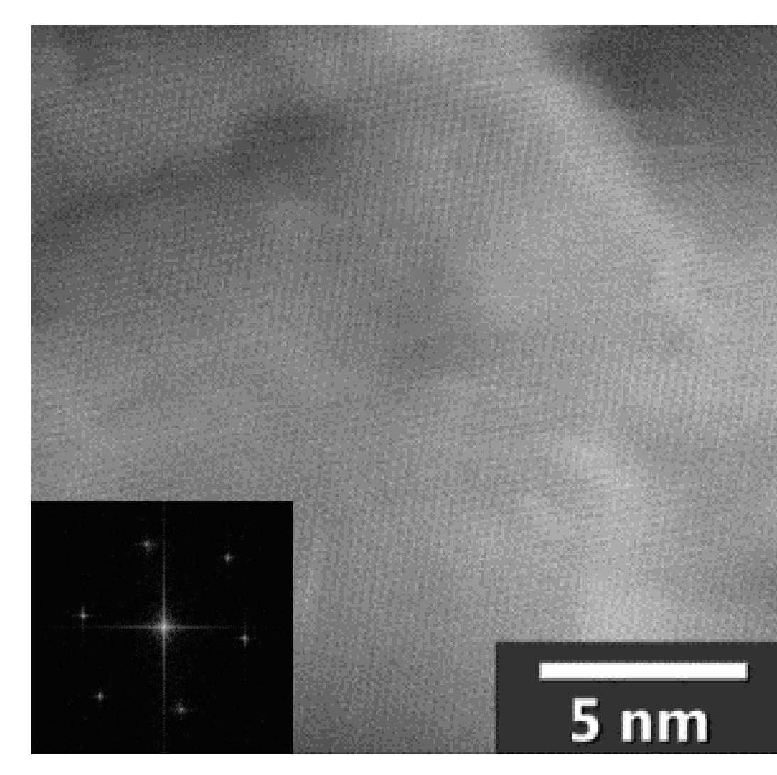
Atomic resolution HAADF STEM image of the same particle and corresponding FFT (inset).
