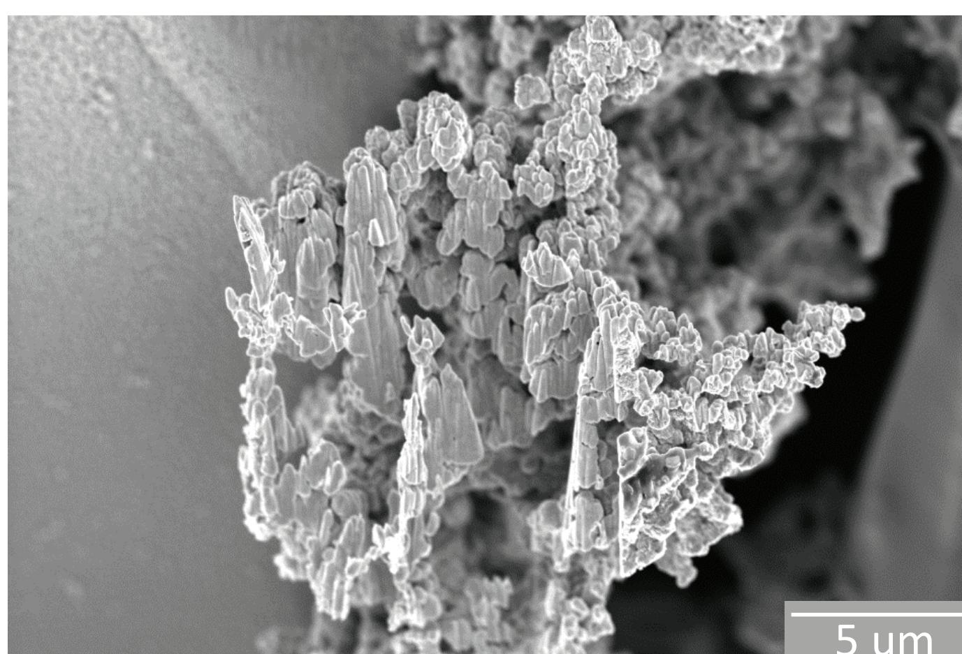
Using basic milling parameters, the particles would fall apart. Here, a regular cross section pattern was used at 30kV and 2.5nA with no adjustment made to the standard FEI Si material file. Overlap 50%, 50%.
