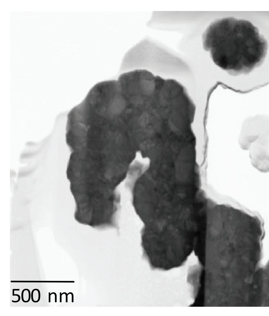
BF STEM image of final thinned (80 nm thick), electron transparent Rh-alloy particle taken in an FEI Titan TEM at 200kV.
