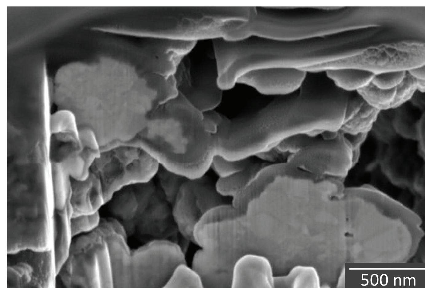
Using the beam path as visual feedback, beam overlap was decreased until a smooth cut was observed. Here, beam overlap is -25%, 0%. At this overlap setting, the particles milled evenly and stayed intact.
