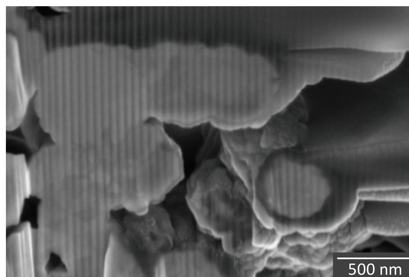
Here, the beam current was lowered to 80pA. Additionally, beam overlap was adjusted to -200%, 0%. At this extremely low X overlap setting, you can actually see the beam path as evidenced by the vertical lines running through the material.
