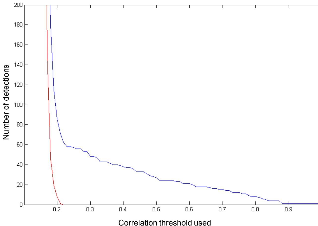
We can see that the detections from noise start when the correlation threshold has a value of about .22
