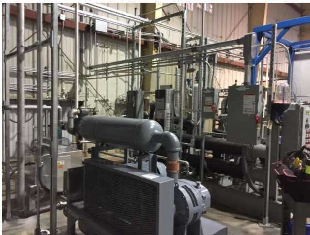
Exhibit 10. Picture of permeate blower installed at 0.1 MWe bench scale skid
