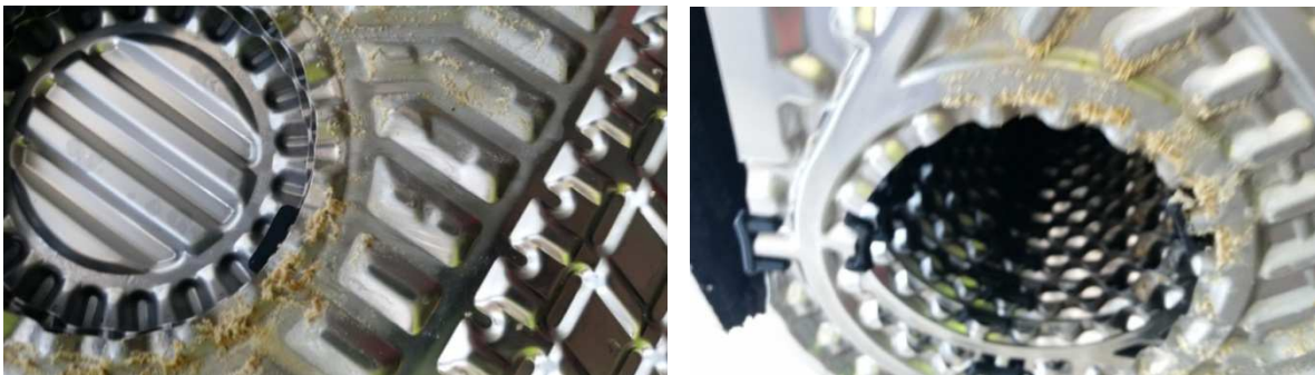
Exhibit 43. Picture of Heat Exchanger Fouling
