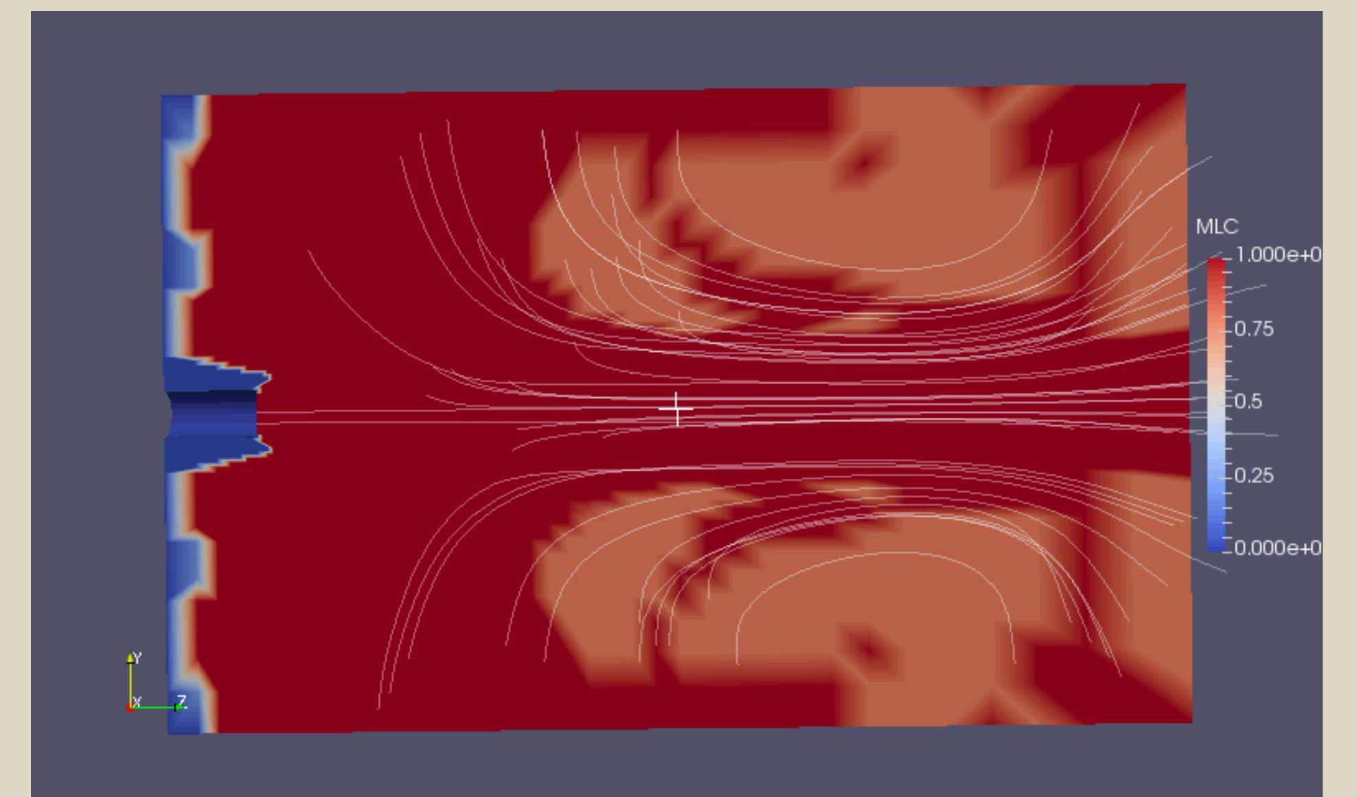
Plot of the degree of turbulent anisotropy in an open jet simulation as calculated from the RF's. Red regions are high anisotropy blue low regions. Stream Lines are overlaid to show flow. Results currently do not appear correct.
