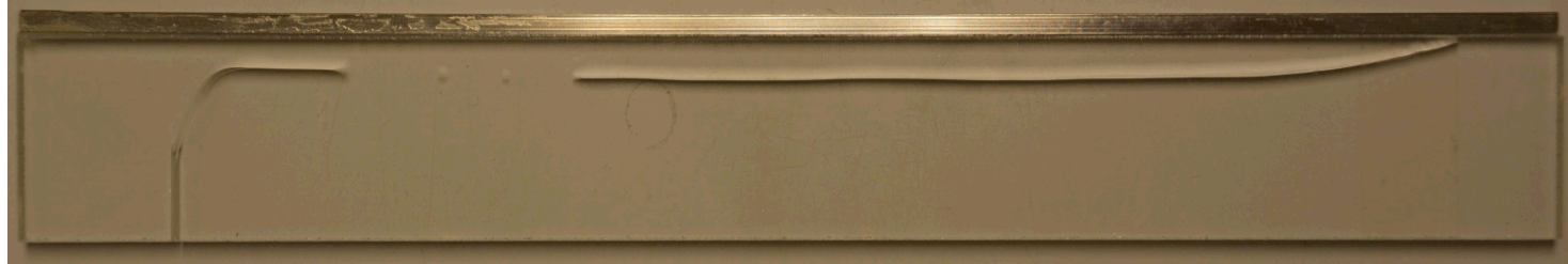
Experimentally observed crack path
