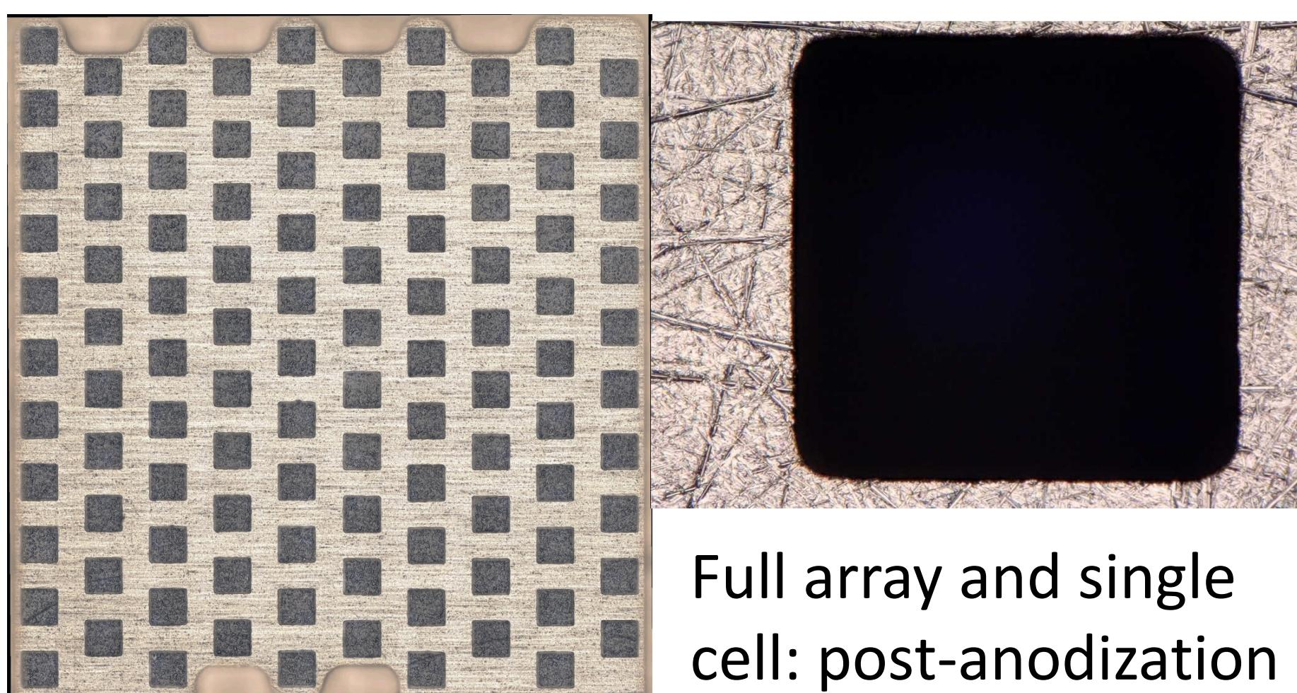
Full array and single cell: post-anodization
