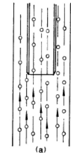
$V_{SAMPLE} = V_{STACK}$
