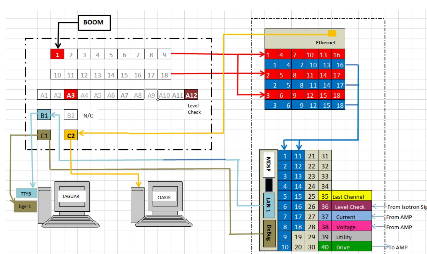
This diagram shows the **cable connection** between the **control CPU**, the **boom** (external liaison between the transducer and the signal conditioner), and the actual **signal conditioner** itself (OASIS).
