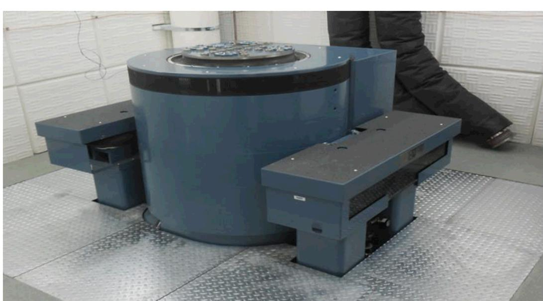
Here is a pictorial representation of a machine used for vibration testing. This device is called a "shaker". It is used to **implement excitation** into a structure at a specified control point.
