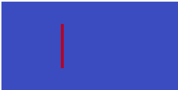
Initial crack/damage in specimen
