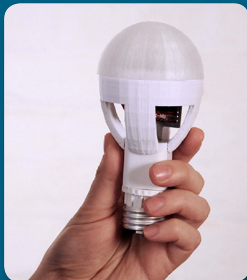
A Wi-Fi-enabled lightbulb with modifiable firmware.
